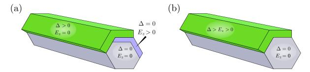
Figure 1: (a) A schematic representation of the experimental setup in Ref. [8]. The system is a heterostructure consisting of three parts: a semiconducting nanowire, an s-wave superconductor as well as a magnetic insulator. (b) Effective model of the same, a semiconducting nanowire coupled to an s-wave superconductor which features a Zeeman term.
