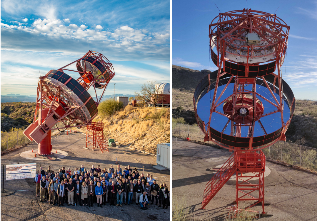
Figure 1. ( Left ) The inauguration of the pSCT at FLWO on January 17, 2019. ( Right ) A picture of the pSCT showing the segmented primary mirror from the front, segmented secondary mirror from the back, and the camera access tower, which enables the maintenance of the camera positioned between primary and secondary mirrors in the Schwarzschild-Couder OS.
