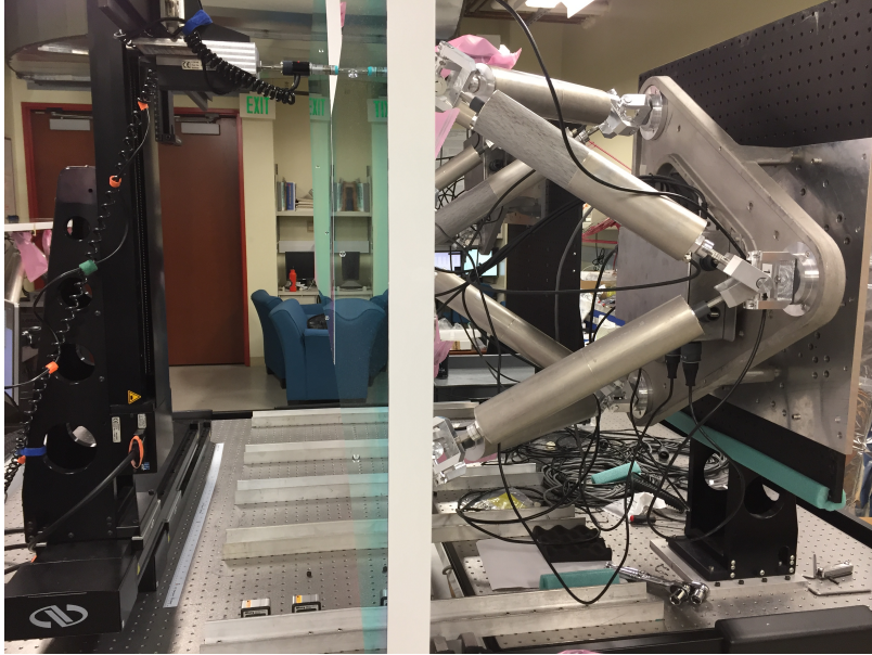
Figure 6. Illustration of the MPES calibration setup in the lab, with an edge-on view of two mirror panels. The white vinyl side of one mirror panel is placed vertically across the middle of the frame of this picture. The two MPMs are mounted vertically. The mounting triangle and the actuators of one panel are visible on the right-hand side of the picture. The CMM with mechanical touch probe is shown on the left-hand side of the picture.
