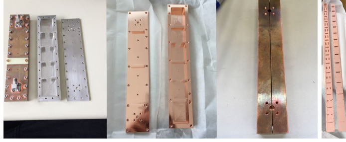
Figure 43. RADES cavities (stainless steel with copper coating) resonating around 8–9 GHz. From left to right: first 5 sub-cavities structure with inductive couplings (non-tunable, used in data-taking 2018 in CAST), alternating inductive- and capacitive-irises sub-cavities structure (non-tunable, used for proof-of-principle of behavior of alternating cavity types), 5 sub-cavities vertical cut structure (tunable, used for cryogenic measurements for the proof-of-principle of tuning), alternating 30-cavities structure (non-tunable, used in data-taking 2020 in CAST). The first three structures are each about 15 cm long, the 4th one is of about 1 m length, see [126, 129, 130] for details.
