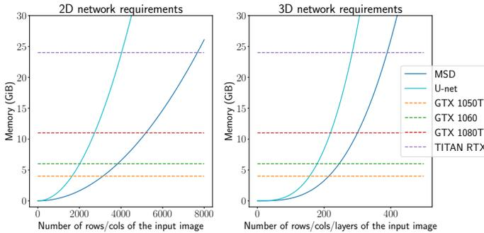
Fig. 5. The required memory to store all intermediate images for applying a 2D and 3D U-net and MSD network as a function of the input image size.
