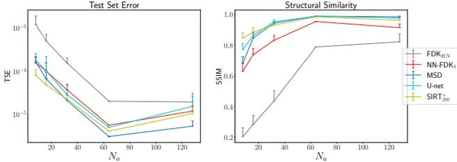
(a) The average and standard deviation of the TSE and SSIM as a function of number of projection angles  $N_a$  computed over 20 randomly generated phantoms Fourshape family.
