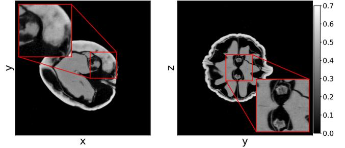
Fig. 4. The  $z = 0$  (Left) and  $y = 0$  (Right) slice of the gold standard reconstruction of the high-dose dataset of the 21<sup>st</sup> walnut with full number of projection angles. The projection data is acquired using the FleX-ray scanner located at the CWI [56].
