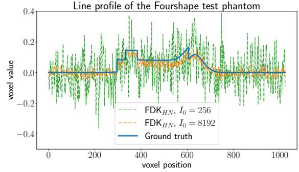
Fig. 8. Line profile through the center of the  $z = 0$  slice of the Fourshape test phantom. We show the ground truth, the profile of the FDK reconstruction with lowest emitted photon count  $I_0 = 256$ , and the profile of the FDK reconstruction with the highest emitted photon count  $I_0 = 8196$ .
