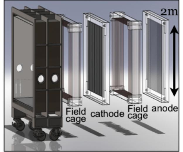
FIG. 31. Design for a first stage  $8 \text{ m}^3$  steel vessel (courtesy of E. Lee, University of New Mexico).
