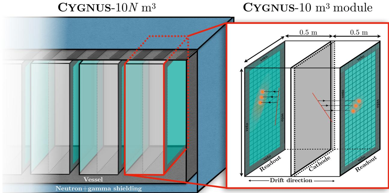
FIG. 1. Schematic of a modular  $N \times 10 \text{ m}^3$  directional detector made up of  $N$  back-to-back TPC modules. Each module would have two readout planes and a central cathode to ensure a short maximum drift distance of 50 cm.
