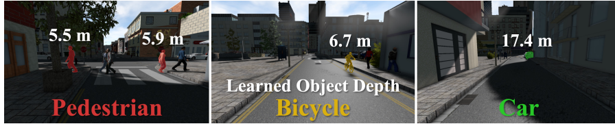
Fig. 7. Driving Test Set Examples and Results. The \text{ODN}_\ell object depth error is -6 and -23 cm for the pedestrians, -10 cm for the bicycle, and -4 cm for the car
