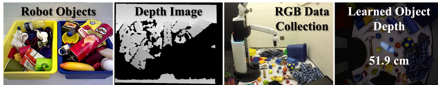
Fig. 6. Robot Experiment Data. HSR view of validation (yellow bin) and test set objects (blue bin) using head-mounted RGBD camera ( left ). Unfortunately, the depth image is missing many objects ( middle left ). However, using 4,400 robot-collected examples ( middle right ), we find that segmentation-based object depth works ( right )
