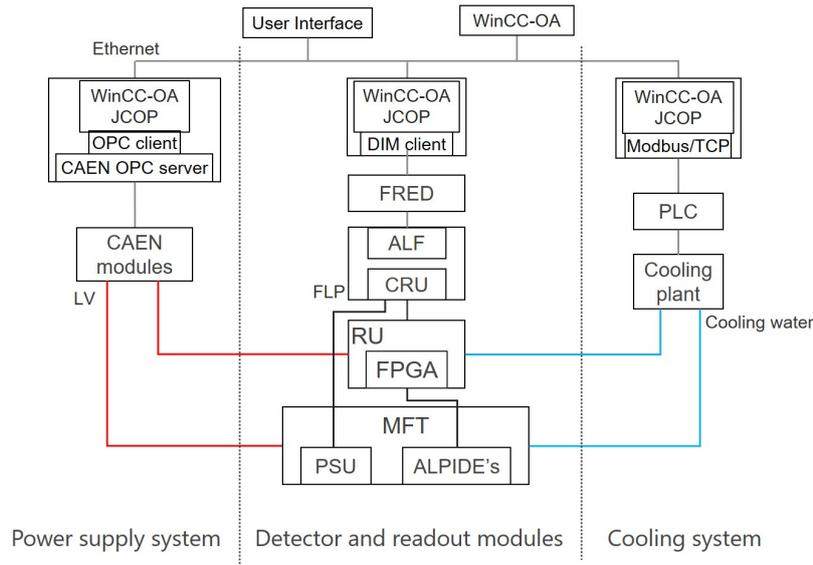
**Figure 5.** Hardware structure of the MFT DCS.
