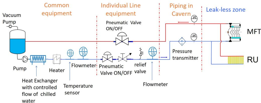
**Figure 7.** Structure of the water cooling system.
