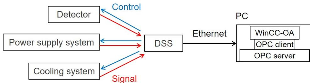
**Figure 12.** MFT Detector Safety System (DSS) layout.
