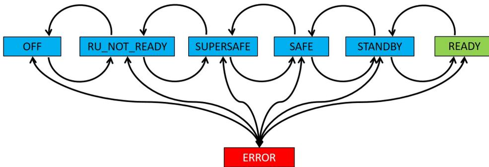
**Figure 10.** State diagram of the MFT top node. The MFT detector is available for physics data taking only in the green READY state. The states with blue boxes mean the status is okay, but not ready for data taking.
