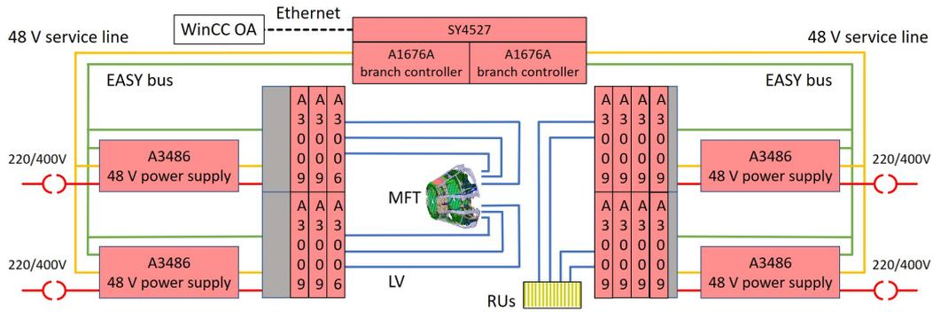
**Figure 6.** Structure of the power supply system.
