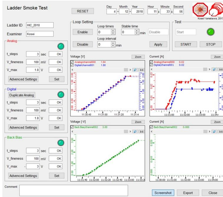
Figure 14. Result of smoke test with back-bias voltage.
