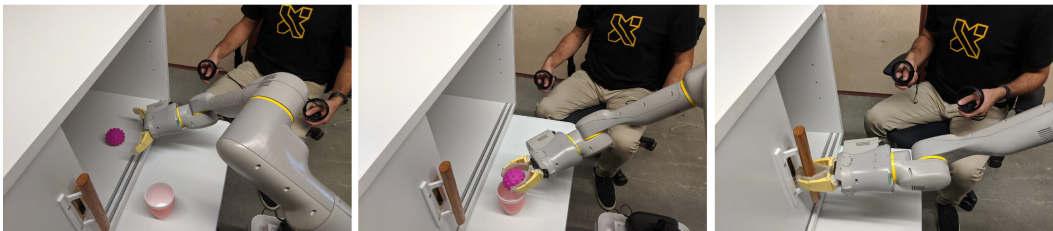
Figure 8: Human operator performing a task of grasping a ball, putting it into a cup, and closing a cabinet door, performed with a teleop system.
