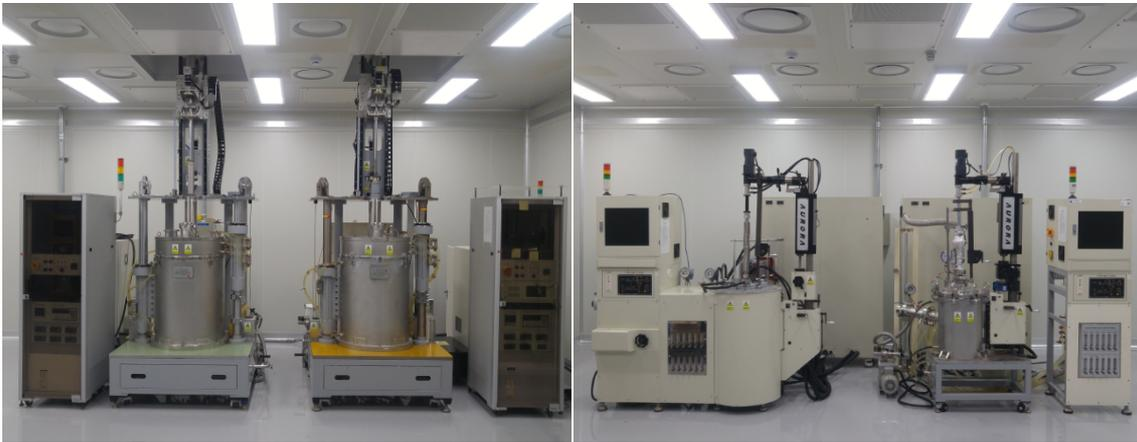
**Figure 1.** Czochralski (left) and Kyropoulos (right) machines in a clean room at the CUP [13].
