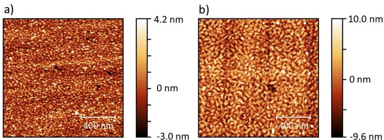
**Figure S1.** AFM image of 30 nm H<sub>2</sub>Pc grown on glass substrate with a) LT condition having rms roughness of 1.9 nm b) RT condition having rms roughness of 2.4 nm
