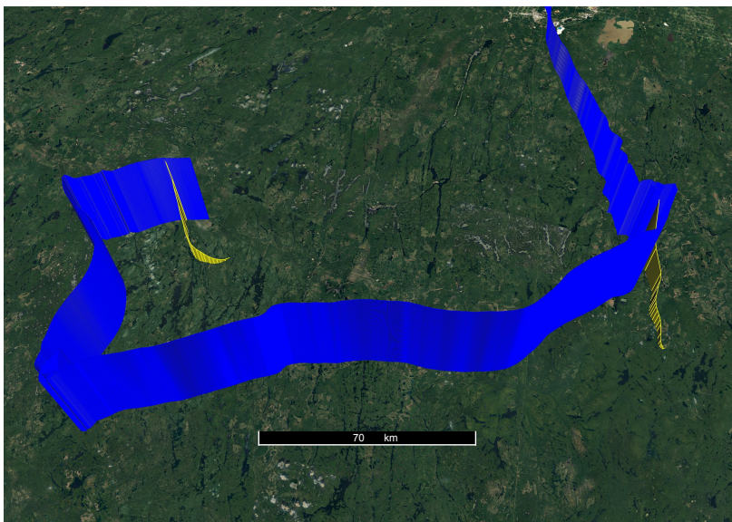
Figure 6. The flight path of the two DRS capsules, while they were attached to SUPERBIT (blue) and while descending independently by parachute (yellow). The trajectory starts near the top right corner of the figure, and continues clockwise. It does not include SUPERBIT’s descent because the main gondola powers down before termination.
