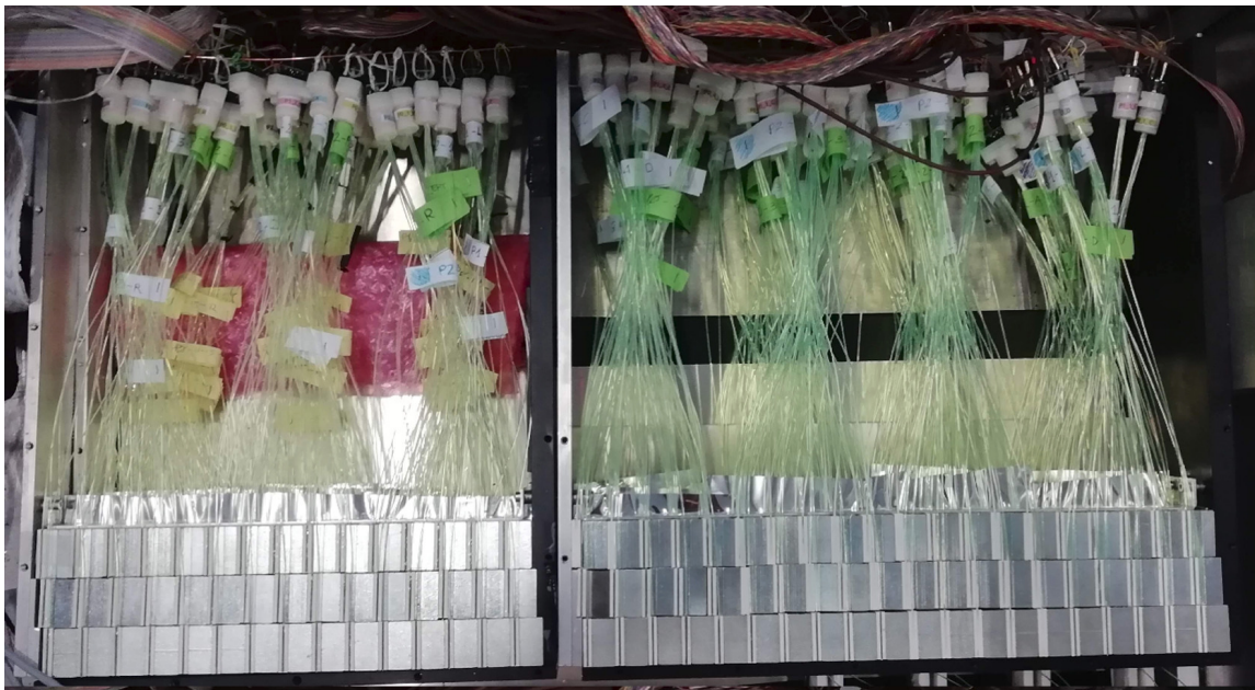
Figure 5. Side view of the prototype with the lateral readout scheme built in 2018. The array of UCMs is on the bottom while SiPMs for the readout of the WLS fibers are on the top at an average distance of \sim 30 \text{ cm} from the bulk.
