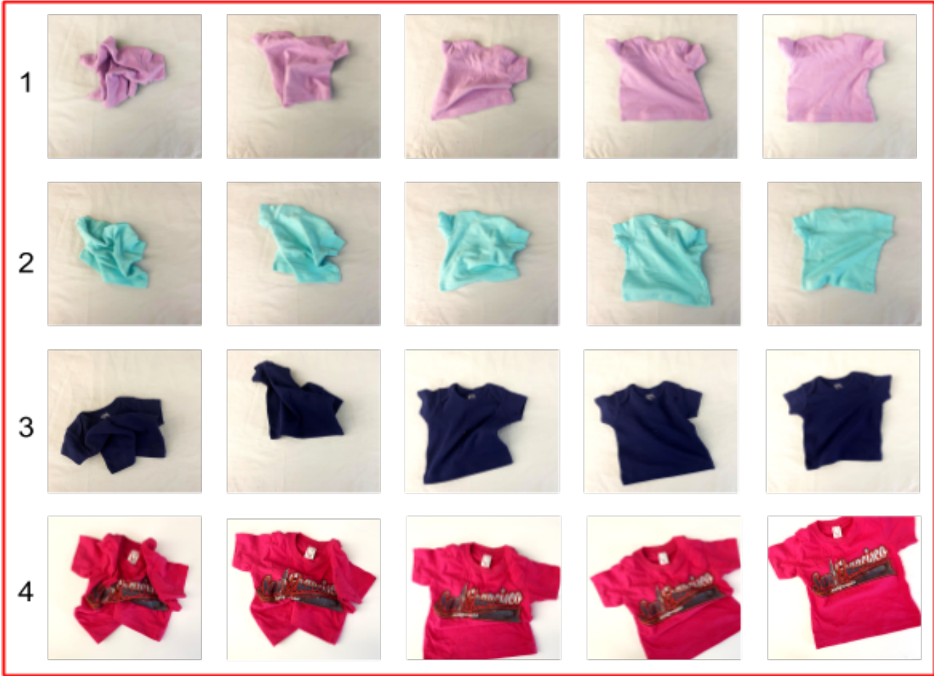
Fig. 11: Additional rollouts of the smoothing task from randomly chosen starting configurations. The learned descriptors are used to locate the corners of the fabric and successively pull them to a reference location in an image of the flat cloth.
