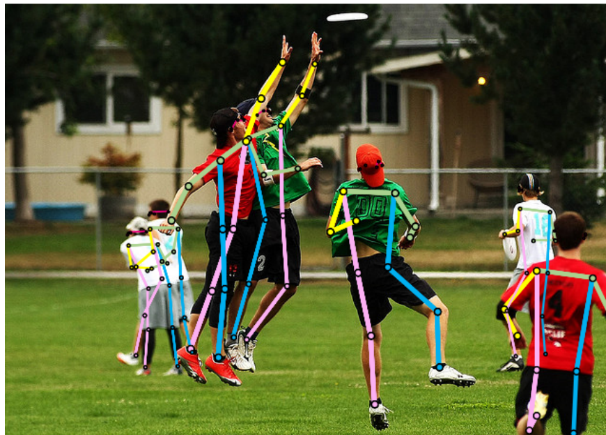
Figure 4: Pose Estimation. Image source [218] The task of pose estimation, specifically multi-person 2D (human) pose-estimation is depicted in the figure. The neural network model predicts the positions of the main joints (keypoints), which are combined with a body model to get the stick-figure like approximations of pose overlaid on the multiple humans in the image. Variants of these techniques have been used to study animal behaviors in scientific settings.
