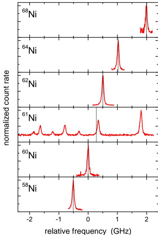
FIG. 1. Spectra of the stable isotopes  $^{58,60,61,62,64}\text{Ni}$  and the radioactive  $^{68}\text{Ni}$  with their center frequency indicated with a vertical line. The count rate is normalized for each isotope, and the frequency is given relative to the center frequency of the reference isotope  $^{60}\text{Ni}$ .
