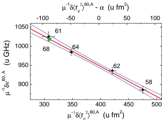
FIG. 2. King-plot analysis of the stable isotopes. The red line is a straight line fit to the black data points taking  $x$ - and  $y$ -errors into account and the  $1\sigma$ -confidence interval is shown as a blue solid line. The top axis is shifted by  $\alpha = 397 \text{ u fm}^2$  to remove the correlation between  $F$  and  $M$ . The green star shows the position of  $^{68}\text{Ni}$ , from which the charge radius is extracted.
