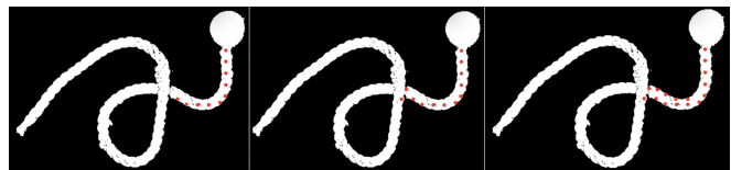
Fig. 14: Nonplanar failure mode. One failure of the analytical-based approach is that the gradient is unclear at areas of overlap in the rope. In this case, the gradient does not follow the rope geometry but rather starts collecting annotations in the opposite direction.
