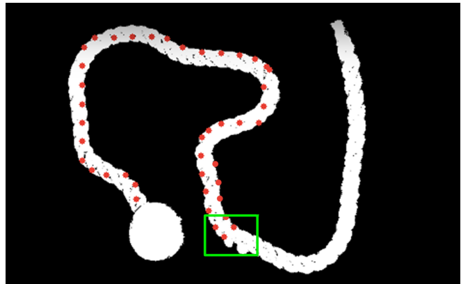
Fig. 13: Rope irregularities failure mode. The nylon rope has non-uniform thickness and fraying. This can confuse the gradient direction, causing the annotations to follow along the curve of an irregular bump rather than along the rope geometry.
