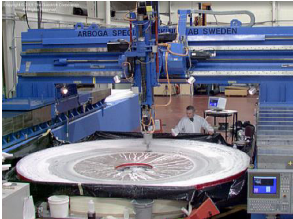
Figure 6.8-2. Collins Aerospace computer-controlled manufacture of 4.2 m SOAR primary mirror (Cox 2018).
