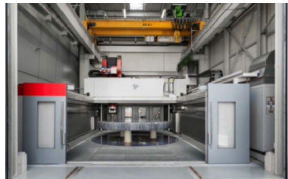
Figure 6.8-1. SCHOTT glass 5 m 5-axis CNC machine center loaded with a 4.5 m glassy Zerodur® blank (Nemati et al. 2017).
