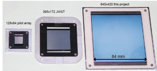
Figure 11.7-3. The Next Generation MSA (right) is over 4× the size of the JWST MSA.
