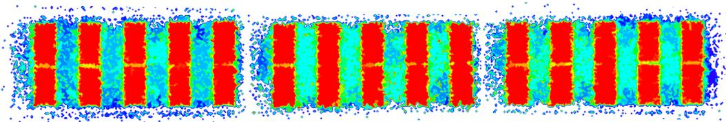
Figure 13: Lateral efficiency maps with a 10 ADC threshold for the three modules. The free surface of the liquid polysiloxane is down in this figure (color version online).
