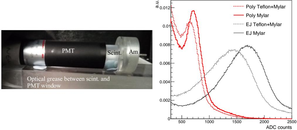
Figure 1: Comparison of light yields with sources. Left: The setup with the Am source, the scintillator cylinder and the photomultiplier. Right: pulse spectra for the Eljen scintillator (thin black) and the polysiloxane one (thick red). Dashed (solid) histograms are obtained with wrapping 1 (2), respectively, see text.
