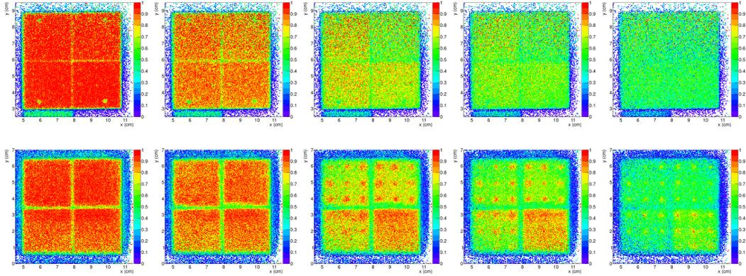
Figure 11: Efficiency maps for increasing thresholds from left to right for the most upstream module using all particle types. The upper row refers to PLAS the lower one to POLY (color version online).
