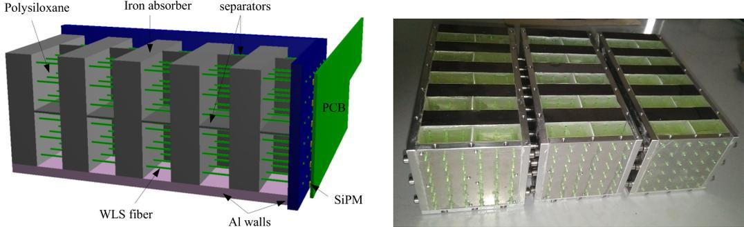
Figure 3: Polysiloxane prototype. Left: annotated sketch of a single module (4 UCMs). Right: a picture of the three calorimeter modules (12 UCMs).
