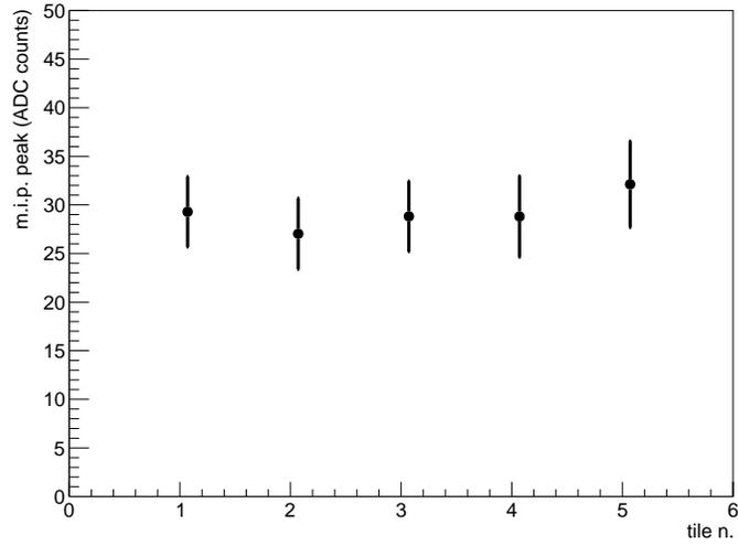
Figure 12: Light yield of the scintillator tiles. Tiles are ordered from 1 to 5 according to their position along the beam direction. Markers represent the means of the most probable values for Landau fits of mip tracks for each tile position in the UCMS, while their spreads is shown by the error bar.
