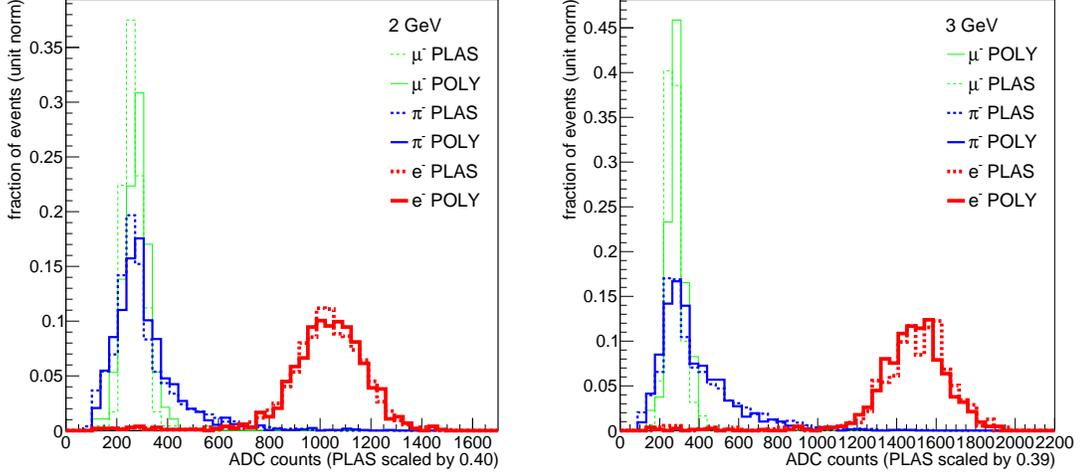
Figure 8: Distributions of the pulse heights for POLY (solid) and PLAS (dashed) at a SiPM bias voltage of 36 V for different particle populations (thicker red line for  $e^-$ , medium thick blue for  $\pi^-$  and thinner green for  $\mu^-$ ) as selected using the Cherenkov counters pair. Left and right plots refer to a beam energy of 2 and 3 GeV respectively.
