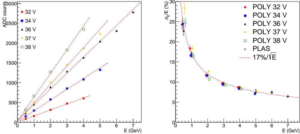
Figure 9: Linearity with electron energy (left) and electron energy resolution (right) for POLY at different values of the SiPM applied voltage.
