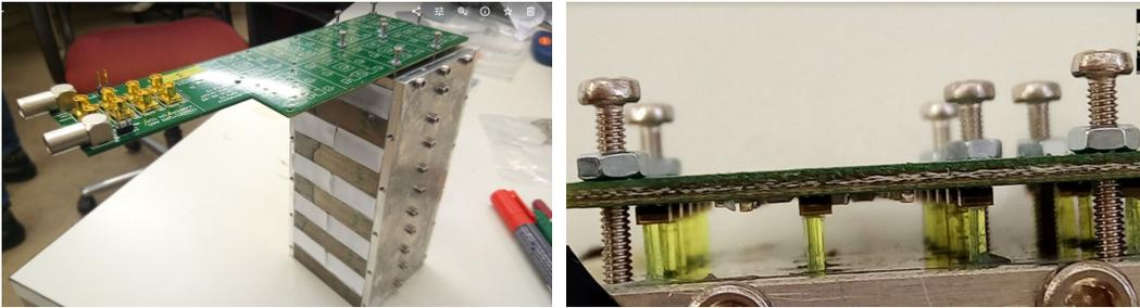
Figure 5: WLS-SiPM coupling. Left: a single module with the PCB installed in the back plane. Right: a close-up lateral view of the PCB with fixing bolts. The Y11 WLS fibers touching the SiPM are visible and could be individually inspected.
