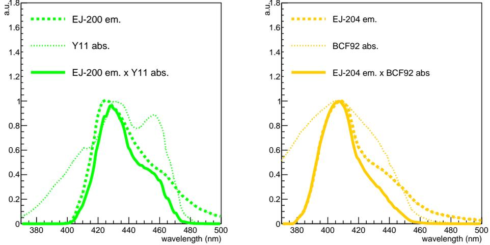
Figure 7: Right: spectral matching between BCF92 fibers and EJ-204 scintillator, equivalent to the PLAS setup. Left: spectral matching between Y11 fibers and EJ-200, corresponding to the POLY setup (EJ-200 emission is very similar to the used polysiloxane-based scintillator).
