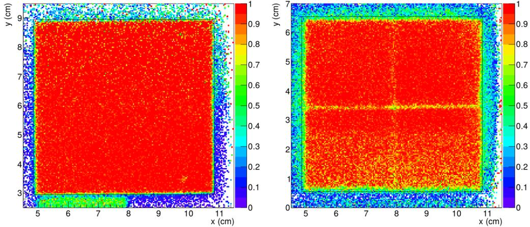
Figure 10: Efficiency map for the PLAS (left) and POLY (right) upstream UCM with a 20 ADC counts threshold (color version online).
