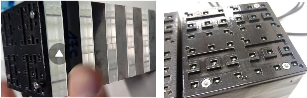
Figure 6: PLAS reference calorimeter. Left: the absorber–scintillator stack before wrapping with black tape. Right: a detail on the 3D-printed mask used to interface the WLS fibers and the SiPM mounted on the PCB.
