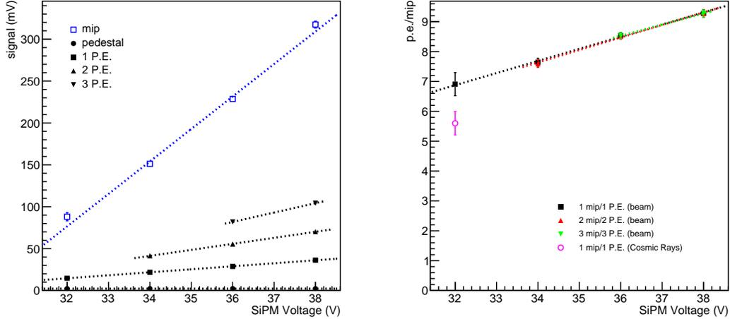
Figure 16: Left: Dependence of the position of 1, 2, 3 P.E. signals (black) and of the mip peak (blue) in ADC counts with the applied SiPM bias. Right: P.E. per mip as a function of the SiPM bias. The measurement obtained with cosmic ray tracks is also reported in magenta (see text for details).
