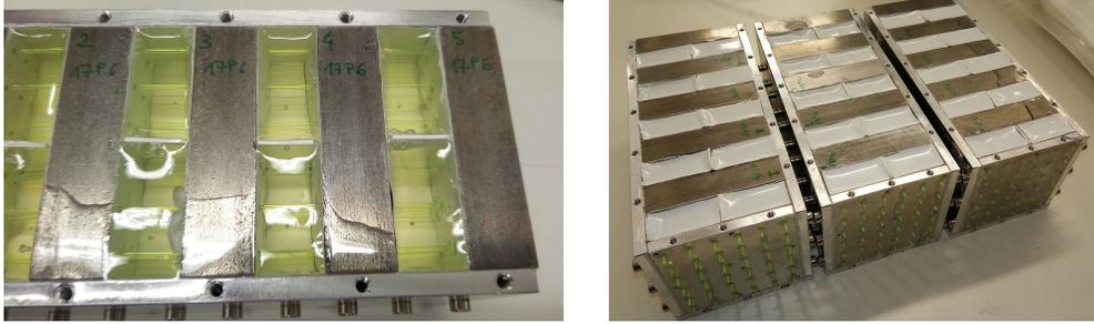
Figure 4: Polysiloxane prototype. Left: close up of scintillator compartments. Right: the full prototype with a white diffuser on the surface face.
