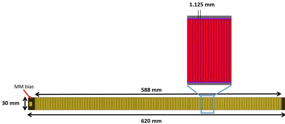
**Figure 3.** Schematic drawing of the position-sensitive Micromegas board.
