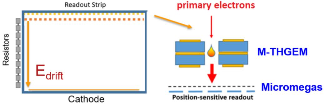
**Figure 2.** Schematic drawing of the novel drift chamber design and of the hybrid Micromegas/M-THGEM avalanche readout.
