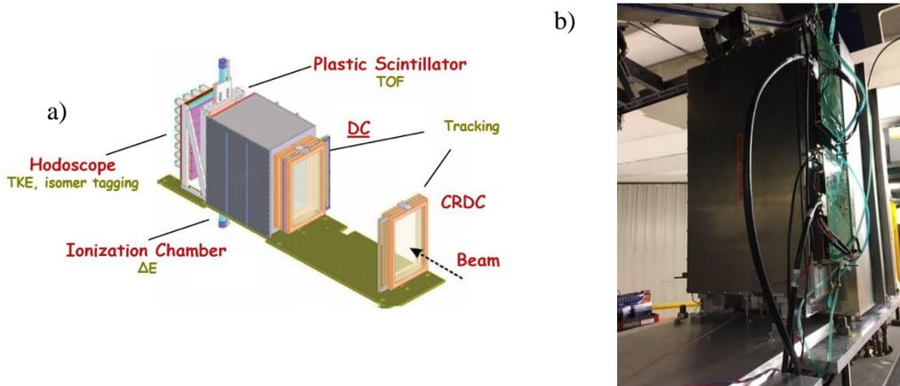
**Figure 8.** Schematic drawing of the detector configuration of the S800 focal plane used for tracking and particle identification (part a) and photograph of the new DC mounted in the s800 focal plane in front of the ionization chamber.
