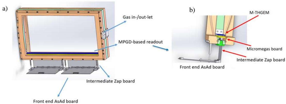
**Figure 1.** Technical drawing of the detector assembling (front view in part a), and detailed of the position-sensitive readout installed in the inner detector frame and associated electronics (side view cut in part b).
