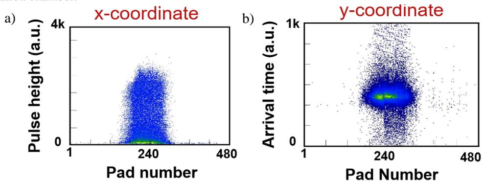
**Figure 9.** Cumulative mapping of the pulse-heights (x-coordinate, part a) and of the signal arrival time (y-coordinate, part b) measured along the Micromegas readout board (pads number) with the  $150\text{ MeV/u } ^{78}\text{Kr}$  beam.
