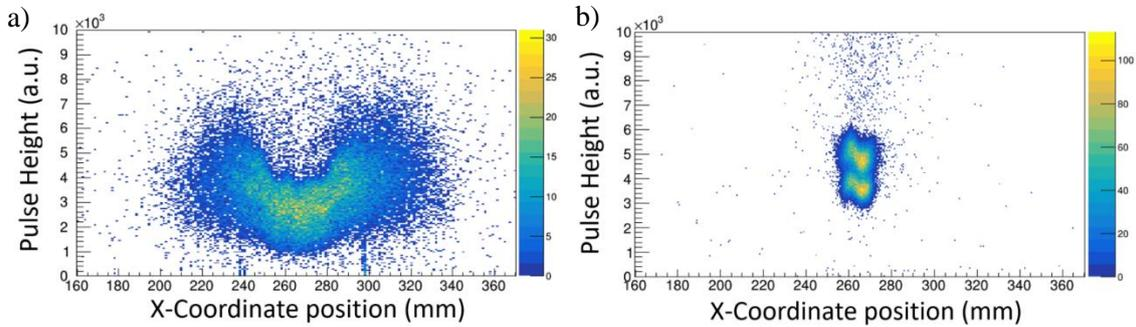
**Figure 6.** Mapping of the pulse height distribution as a function of the particle position along the Micromegas readout for a non-collimated source (part a) and for particles impinging on the narrow selected detector area by using a small Si detector as trigger (part b).
