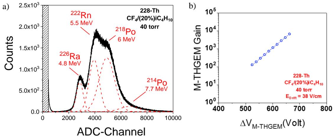
**Figure 5.** Energy spectrum of  $^{228}\text{Th}$  recorded by the Micromegas mesh (part a). Gas gain provided by the M-THGEM pre-amplification element as function of the voltage different applied across each multiplication stage (part b). In both case, the detector operated in  $\text{CH}_4/20\%\text{iC}_4\text{H}_{10}$  at 40 torr (part a). Gas gain of the
