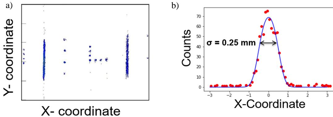
**Figure 10.** Part a: image of the calibration mask obtained by irradiating a large portion of the DC detector area with 150 MeV  $^{78}\text{Kr}$ . Part b: position resolution (0.25 mm sigma) estimated from the processing of a hole in the calibration mask image of part a).
