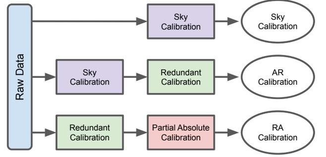
**Figure 15.** Schematic showing the order of operations for three related calibration strategies, similar to that of Li et al. (2018). For AR and RA calibration, the gains from the first step are applied to the data before proceeding to the second step. In addition, the gains derived by redundant calibration have their degenerate modes projected out before proceeding.
