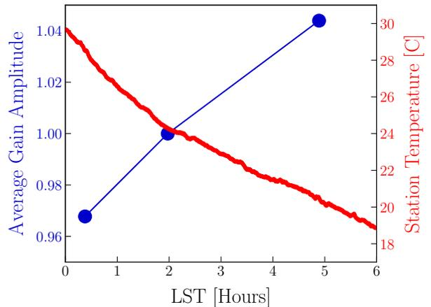
**Figure 14.** The average gain amplitude drift (blue) throughout the 2458098 observing night, derived from three independent calibration fields and normalized to the field at 2 hours. We also overplot the ambient temperature measured by a nearby weather station (red), showing an expected inverse correlation with the gain drift. Using [Equation 3](#) these data yield a gain temperature coefficient of  $-0.031 \text{ dB K}^{-1}$ .
