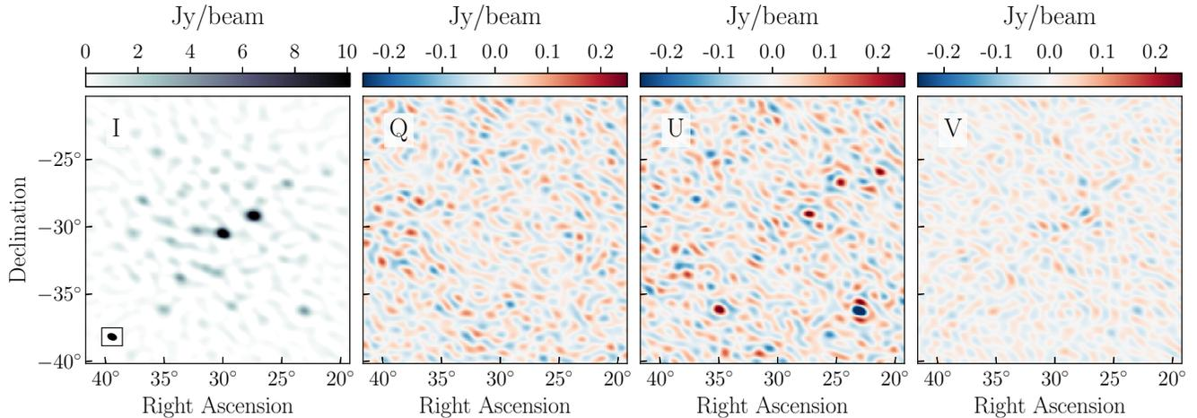
**Figure 6.** Multi-frequency synthesis images (120 – 180 MHz) of the GLEAM-02H field in all pseudo-Stokes I (far-left), Q (center-left), U (center-right) and V (far-right) polarizations. Each image is CLEANed with the same parameters down to 1 Jy, with the CLEAN beam shown in the lower left. Even with no polarization calibration, the observed leakage from I  $\rightarrow$  Q, U & V is a few percent.
