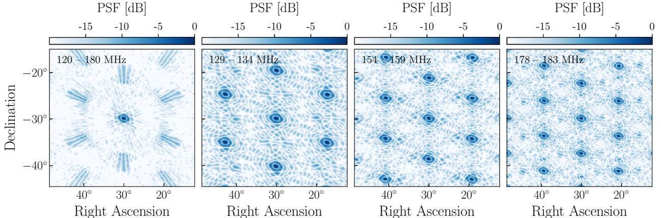
**Figure 7.** The HERA Phase I point spread function (without primary beam correction) from a 5-minute observation across a wide band (left), and a narrow band located in a low-band spectral window (center-left), mid-band spectral window (center-right) and high-band spectral window (right). The grating lobes of the narrow band spectral windows appear in hexagonal patterns reflecting the (un-)sampled  $uv$  spacings on the array, and reach upwards of 50% of the peak PSF response at image-center.
