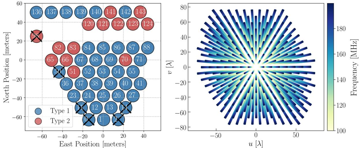
**Figure 2.** **Left:** The HERA Phase I array layout with 56 connected antennas and 50 operational antennas. Antennas determined to be problematic are marked with crosses. **Right:** The corresponding  $uv$  sampling of the array over a 10-minute time window and a frequency range of 100 – 200 MHz, highlighting HERA’s highly redundant  $uv$  sampling. The color gradient represents independent  $uv$  samples throughout the total bandwidth.
