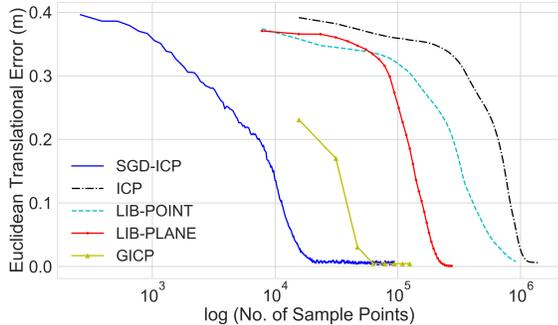
Fig. 1. Comparison of the amount of points needed by different methods to achieve the same level of performance. The amount of points processed is shown in log-scale on the X-axis and clearly shows how SGD-ICP achieves the same result as other methods in roughly a single pass through the point cloud which contains 15646 points.
