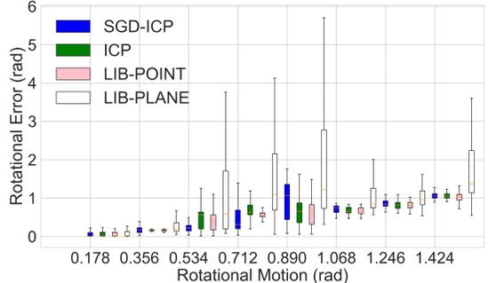
Fig. 2. Comparison of the ability to handle errors in the initial transform by the different methods. The two plots show sensitivity to translational error (left) and rotational error (right). The X-axis shows the amount of error in the initial transform in meters and radians respectively.
