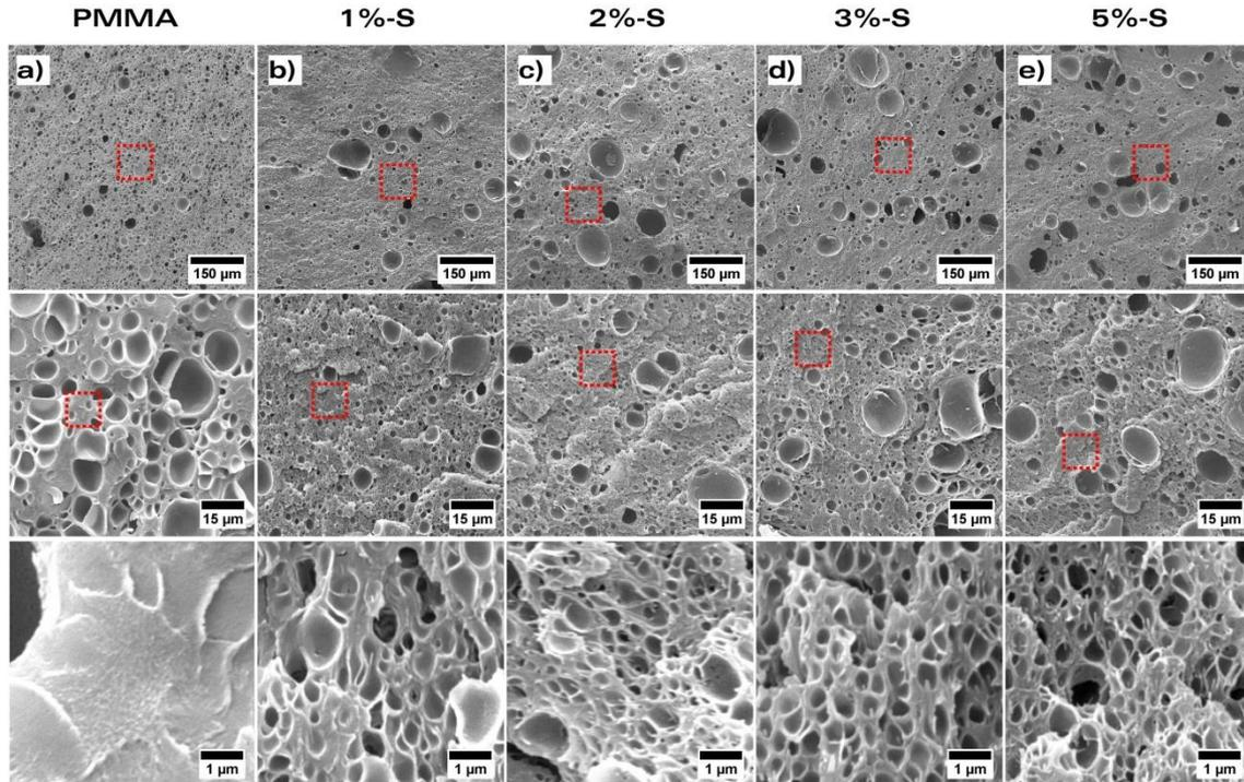
**Figure 1.** SEM images of the samples produced at a foaming temperature equal to 40 °C and foaming time equal to 5 minutes: a) PMMA, b) 1%-S, c) 2%-S, d) 3%-S and e) 5%-S. The second and third rows show images of the same materials at increased magnification.
