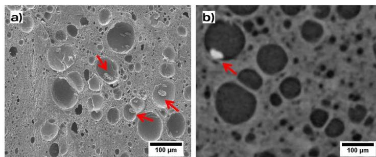
**Figure 8.** Example of aggregates inside the microcellular pores (red arrows): a) SEM micrograph of the cellular material 5%-S with relative density close to 0.5 and b) reconstructed tomography of the cellular material 2%-S with relative density around 0.5.
