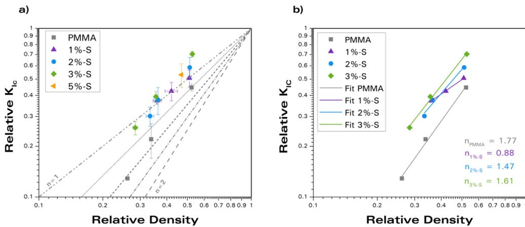
**Figure 10.** a) Relative fracture toughness ( $K_{IC}$ ) of the cellular PMMA and the nanocomposites as a function of the relative density with contours predicted by equation (7) for  $K = 1$  and varying  $n$  values ranging from 1 to 2; b) Fits of the relative modulus according to equation (7) and resulting fitted  $n$  values.
