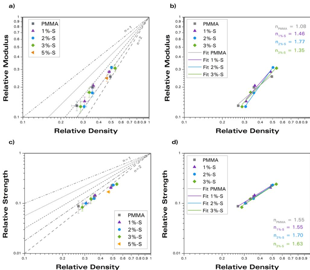
**Figure 4.** a) Relative modulus of the cellular PMMA and the nanocomposites as a function of the relative density with contours predicted by equation (7) for  $K = 1$  and  $n$  values ranging from 1 to 2; b) Predicted trends by fitting equation (7) to the relative modulus data with corresponding  $n$  values; c) Relative compressive strength of the cellular PMMA and the nanocomposites as a function of the relative density with contours predicted by equation (7)
