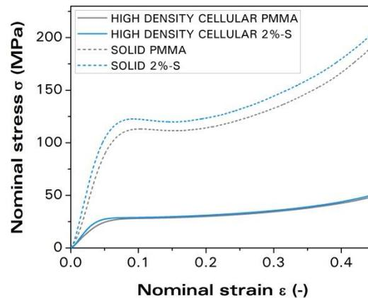
**Figure 2.** Example of stress-strain curves obtained during uniaxial compression of the solid materials and cellular samples with high relative density (around 0.5) based on the PMMA and 2%-S material systems.
