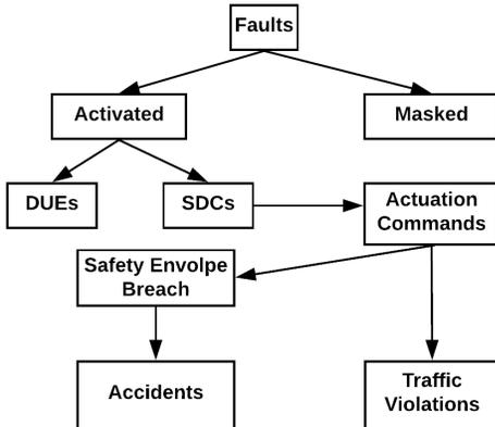
Figure 4: Ontology model for fault manifestation in AVs
