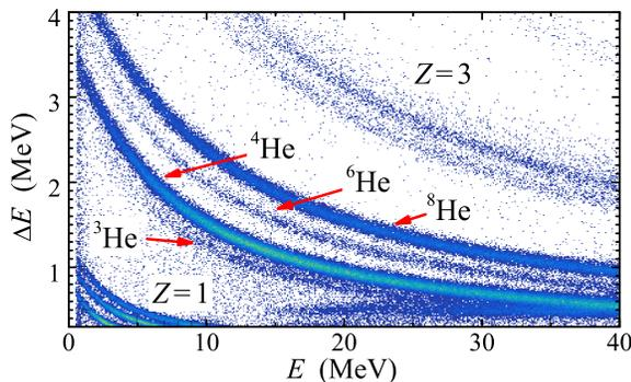
FIG. 3: The  ${}^3\text{He}$  recoil identification. The accurate thickness mapping of the  $\Delta E$   $20\ \mu\text{m}$  detectors was made before the beam exposition to get reliable  ${}^3\text{He}$ - ${}^4\text{He}$  separation.
