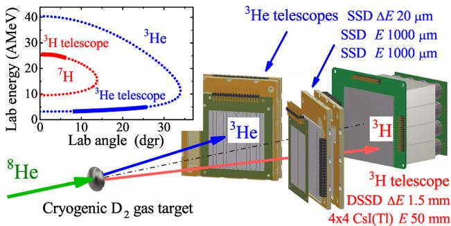
FIG. 1: The sketch of the experimental setup. The inset shows kinematical conditions for the  $^2\text{H}(^8\text{He}, ^3\text{He})^7\text{H}$  reaction at 26 AMeV.
