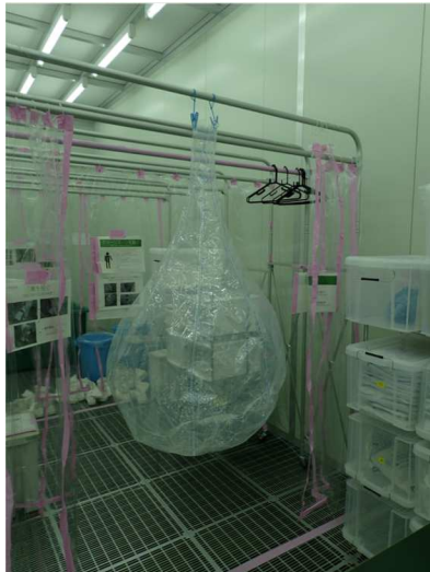
Fig. 8 Test-size scintillation balloon in a clean room (left) and water tank with ultraviolet light (right). The balloon in the left figure is filled with air, while that in the right figure is filled with water.
