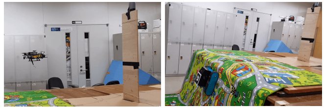
(a) The UAV attaching a tether to a pole-like structure by flying winding the tether attached by around it. (b) The UGV climbing a cliff by winding the tether attached by the UAV
