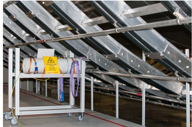
Fig. 5 The ^{60}\text{Co} source used to increase the gamma radiation at the MS. The upper panel is a schematic of the source (in the “closed” configuration). In the bottom panel, the source can be seen installed next to the air-coils, beneath the MS vessel.
