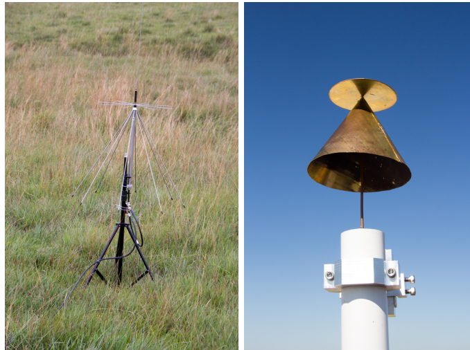
Fig. 2. The discone antennas used in this work. Left: D130J wire discone. Right: custom solid discone.
