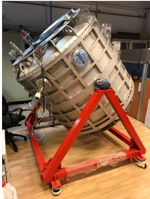
Figure 4: Closed cryostat under test
