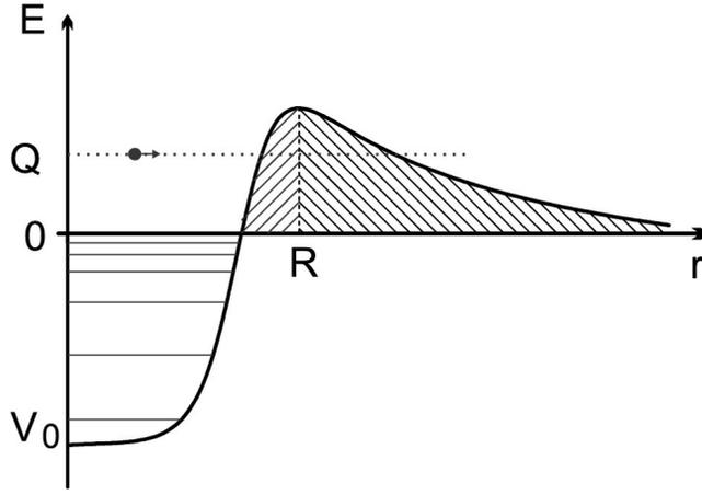
Figure 2: A one-dimensional schematic view of the particle emission process through the Coulomb barrier. Adapted from Ref. [21].
