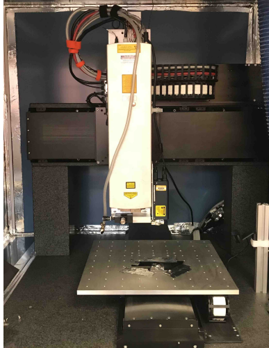
Figure 11. The laser machining setup at the University of Michigan is shown above. The laser has a power of 20 W, and the stages have a speed of 60 mm/s with micron accuracy, allowing for large-format, rapid wafer production.
