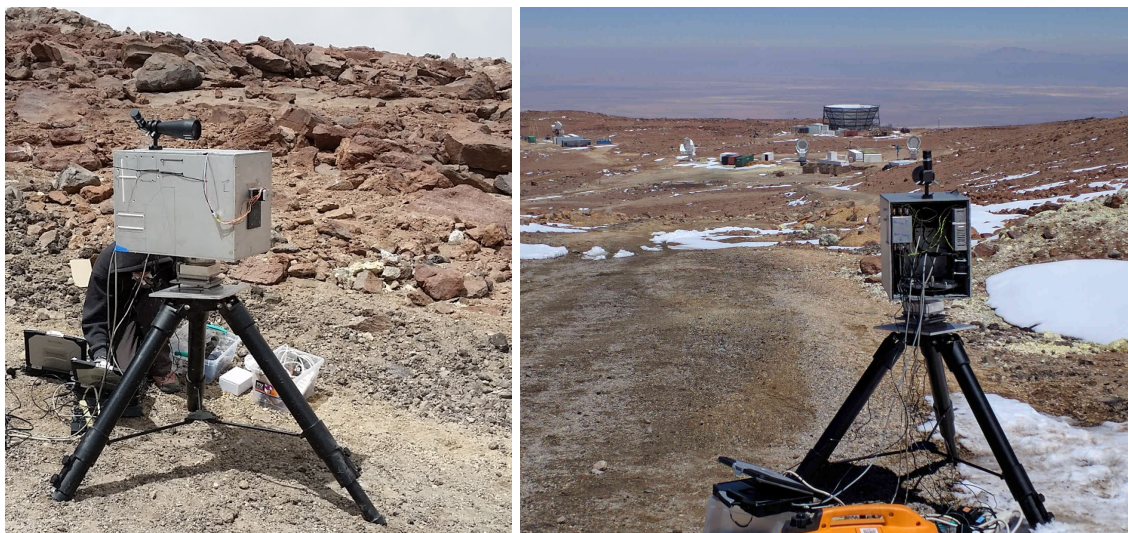
Figure 3. Left : The full polarization calibrator setup at the POLARBEAR site in the Atacama Desert, Chile. Right : The calibrator pointed towards the POLARBEAR telescope.
