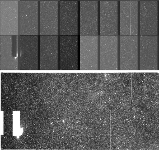
**Figure 3.** Upper: an example of a raw frame from the Transit field where 16 readouts are obvious due to differing bias levels and over-scan. Lower: the preprocessed image from this example; two white regions in the left-lower readout mask the damaged part of CCD.
