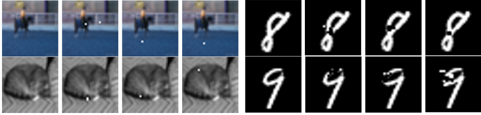
Fig. 7: Some adversarial examples found by our tool L0-TRE while generating test cases for high neuron coverage on MNIST and CIFAR-10 DNNs
