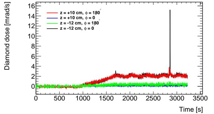
Figure 7: Example of dose rates in diamond detectors, due to beam losses during the initial vacuum scrubbing by the positron LER beam at about 18 mA. This data sample corresponds to about one hour; the initial beam injection and the top-off at intervals of 4 minutes can be clearly identified. Occasional large beam loss spikes (so called “beam-dust events”) are seen in coincidence by more than one diamond detector.
