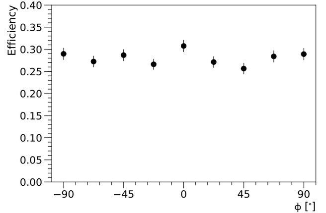
Figure 101: Efficiency of neutron selections in TPCs described in Table 35 versus recoil polar angle  $\theta$  (upper plot) and azimuthal angle  $\phi$  (lower plot) in both TPCs in simulated nuclear recoils. Each point is a ratio of the number of events at a given reconstructed  $\theta$  and  $\phi$  passing all neutron selections to the total number of events. The error bars show statistical uncertainties only.
