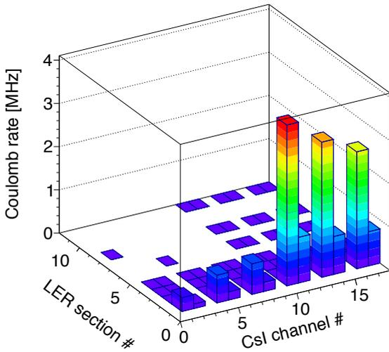
Figure 53: Crystals hit rate as function of the Coulomb scattering LER ring loss position. The rings have been divided in 12 sections, each of 250 m. The dashed lines are fits.
