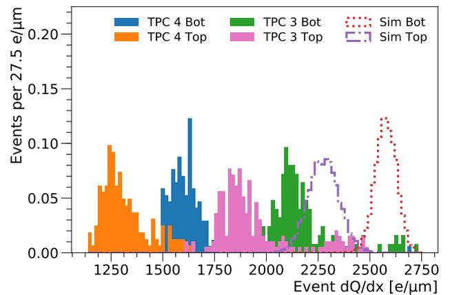
Figure 33: Histograms of the ratio of detected charge to track length [ $dQ/dx$ ] for events from internal  $^{210}\text{Po}$  calibration alpha sources in experimental and Monte Carlo data. The vertical axis shows the total number of events from both sources, normalized to 1, for TPC 3, TPC 4, and Monte Carlo separately. The mean value of each peak is then used as an input in calculating the correction factors shown in Table 15.
