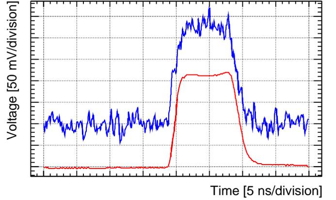
Figure 10: Snapshot of signal from a diamond channel generated by  $\alpha$  particles, processed by a fast amplifier and a large bandwidth oscilloscope. The upper line is the signal due to a single event, while the lower, smoother line is the result of an average of 1000 events.
