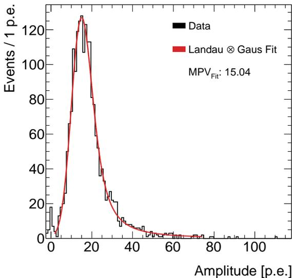
Figure 23: Distribution of the signal amplitude for cosmic muons in one CLAWS detector. The most probable value ( $MPV_{Fit}$ ), used for the detector-to-detector calibration of the CLAWS system, is determined by a fit with a Landau convolved with a Gaussian. The fit result is  $15.0 \pm 0.2$  p.e.
