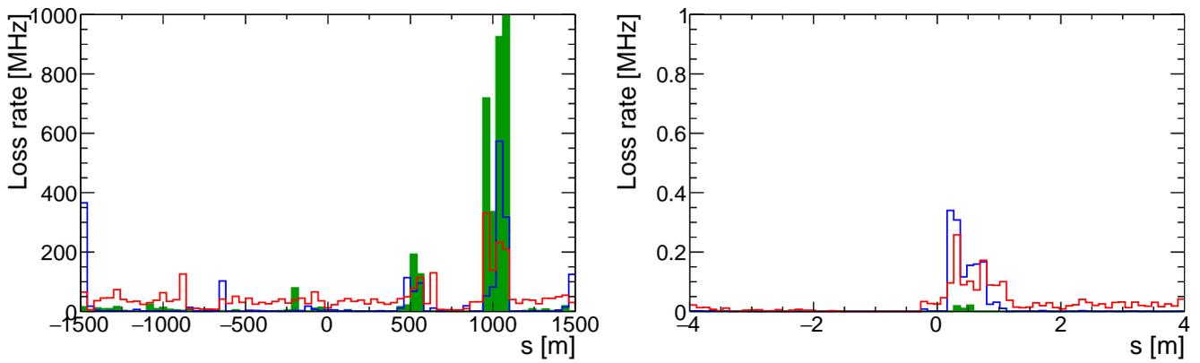
Figure 38: (color online) HER loss rate distributions from SAD, with contributions from Touschek (solid green), Coulomb (blue) and bremsstrahlung (red). For the HER, positive  $s$  is upstream. Upper: full ring. Lower: Interaction region only.
