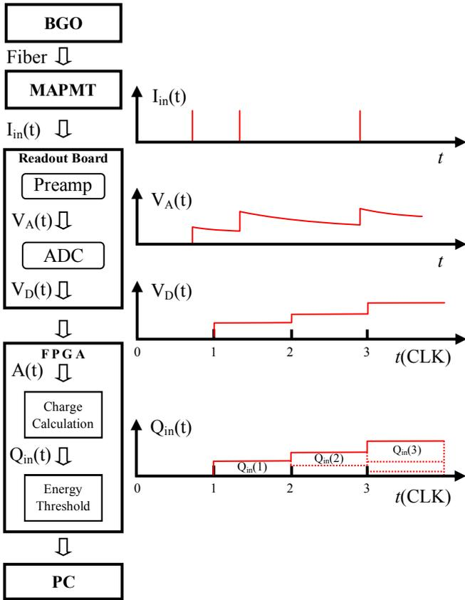
Figure 18: Signal-flow graph of the BGO detector system.
