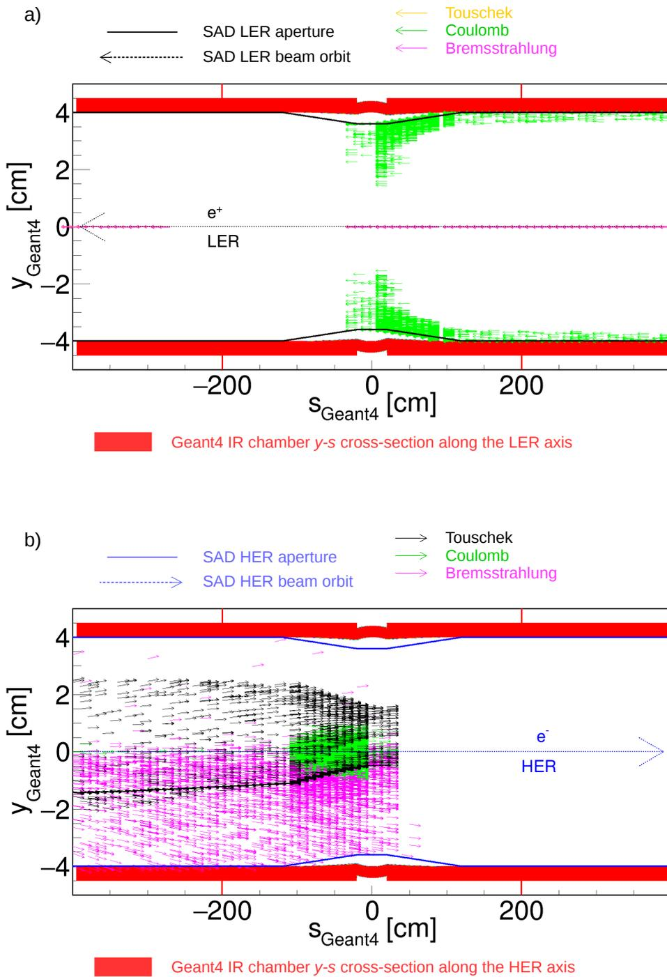
Figure 48: (color online) Geant4 IP chamber vertical cross section versus (a) the LER axis and (b) the HER axis,  $s_{\text{Geant4}}$ , with the SAD aperture and beam orbit overlaid. The arrows indicate the electron beam direction and particles lost direction due to Tauschek, bremsstrahlung, and Coulomb.
