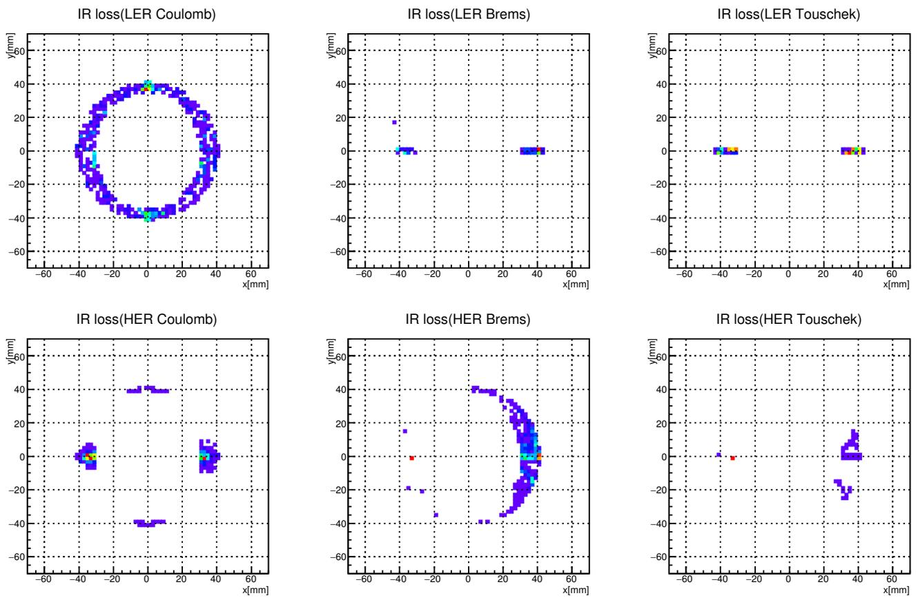
Figure 40: The x-y distribution of the particles lost within  $\pm 4$  m of the IP.
