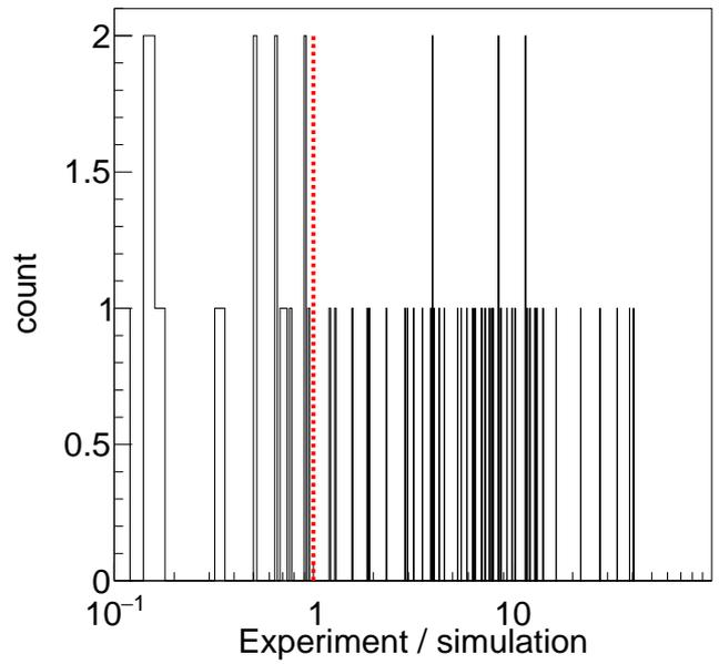
Figure 115: Ratio of the measured and simulated integrated dose in four of the BEAST II detector systems, with periods of injection excluded.
