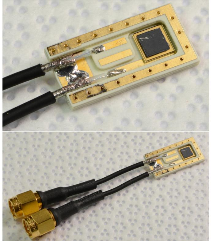
Figure 6: (color online) One of the ( $4.5 \times 4.5 \times 0.5$ ) mm<sup>3</sup> diamond sensors, mounted in its package with short, thin coaxial cables and SMA connectors. In the enlarged image, the golden wire bonds are visible on the upper electrode, deposited on the transparent diamond crystal.
