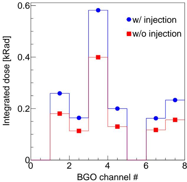
Figure 118: Integrated experimental dose per channel for the BGO system, with periods of injection included (with injection) and excluded (without injection).
