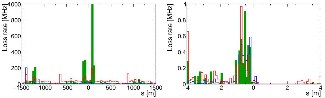
Figure 37: (color online) LER loss rate distributions from SAD, with contributions from Touschek (solid green), Coulomb (blue) and bremsstrahlung (red). For the LER, positive  $s$  is downstream. Upper: full ring. Lower: Interaction region only.
