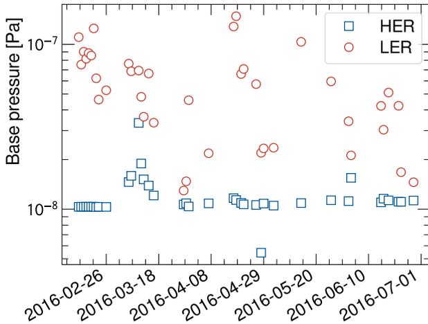
Figure 79: (color online) Dynamic and static pressure measurements: base pressure measured as a function of date. Red circles represent LER measurements, while blue squares represent HER measurements.
