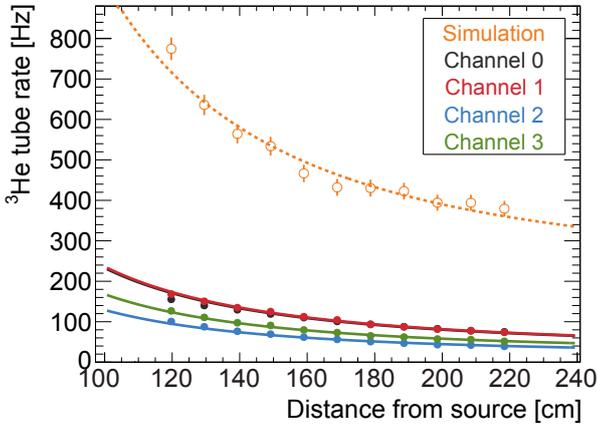
Figure 28:  $^3\text{He}$  tube rate vs distance from thermal neutron source with fits to Eq. 21, showing relative and absolute efficiency of  $^3\text{He}$  tubes
