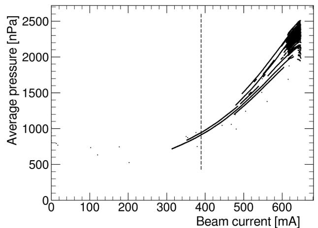
Figure 78: Dynamic and static pressure measurements: example of P-I curves on a full day. Data shown are for the LER on 2016-05-08. The dashed line represents 60% of the maximum current value. Beam injection periods are removed.
