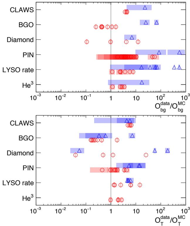
Figure 67: (color online) Experimental/simulated observable ratios derived from Touschek size-sweep runs as described in Sec. 6.3.1. Each point corresponds to a set of LER (red circles) or HER (blue triangles) size sweep runs for a single channel. Shaded bars indicate the errors on the ratio derived from the fit errors to the heuristic.
