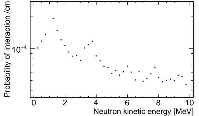
Figure 29: Simulated fast neutron interaction probability per cm as a function of neutron energy in 1 atm of pressure of the 70% helium and 30% carbon dioxide TPC target gas at room temperature. Below 2 MeV, the scattering is almost exclusively elastic.
