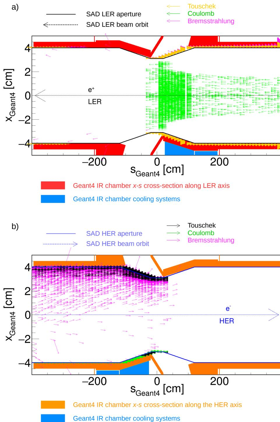
Figure 47: (color online) Geant4 IP chamber horizontal cross section versus (a) the LER axis and (b) the HER axis,  $s_{\text{Geant4}}$ , with the SAD aperture and beam orbit overlaid. The arrows indicate the positron beam direction and particles lost direction due to Touschek, bremsstrahlung, and Coulomb.
