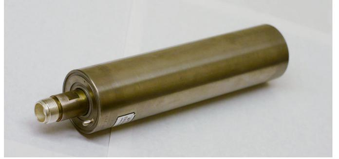
Figure 24: Photograph of a  $^3\text{He}$  tube.
