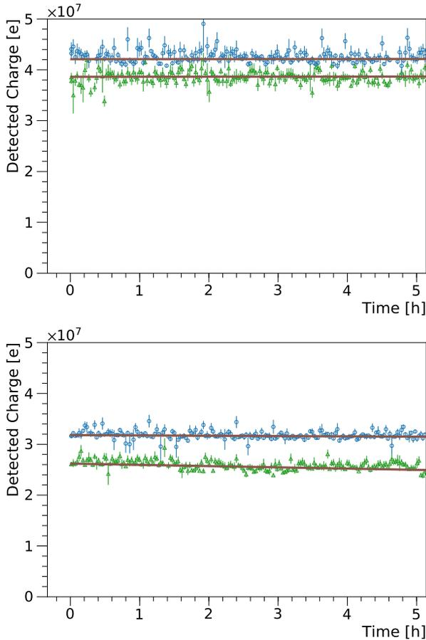
Figure 31: (color online) Detected charge of alpha particle calibration events in TPCs 3 (upper plot) and 4 (lower plot), versus time. The blue circles in each plot correspond to the bottom  $^{210}\text{Po}$  source, corresponding to the source at smaller drift distance, and the green triangles correspond to the top calibration source at larger drift distance. Each line represents the fit of the change of energy over time of events from each internal calibration source.
