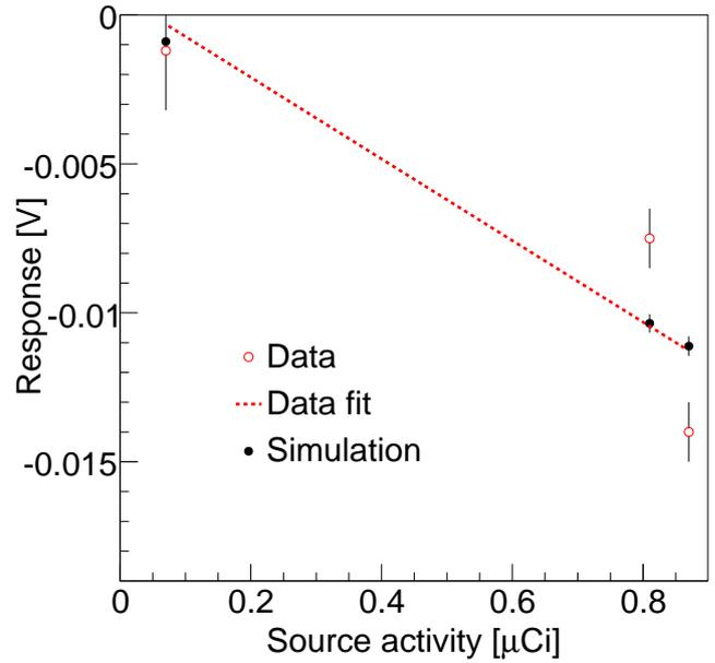
Figure 54: PIN calibration: output versus source activity for a PIN diode with both experimental (open circles) and simulated (closed circles) data.
