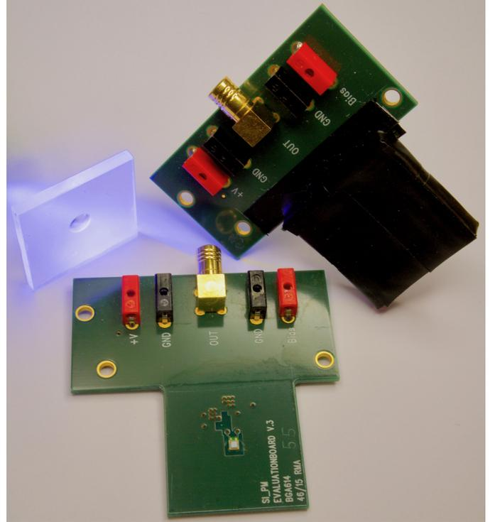
Figure 20: Photograph of one CLAWS detector (top right) as well as of the main components, a  $30 \times 30 \times 3 \text{ mm}^3$  scintillator tile (top left) and the PCB with photon sensor, preamplifier and connectors for power and signal (bottom middle). The plastic scintillator tile, wrapped in reflective foil, is mounted with the dimple located on top of the photon sensor on the PCB. The full detector is enclosed in light-tight wrapping.
