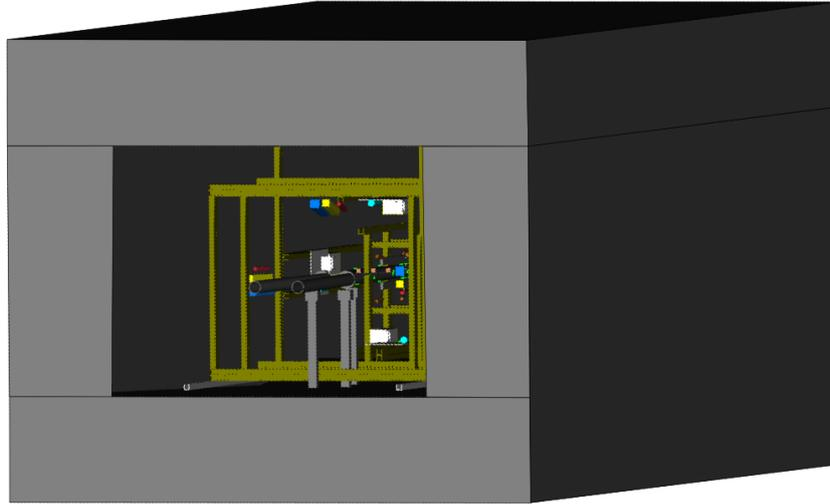
Figure 43: (color online) Color-coded visualization of the Geant4 model. The largest structure is a cement shield, which surrounds the BEAST II setup and SuperKEKB IP chamber.
