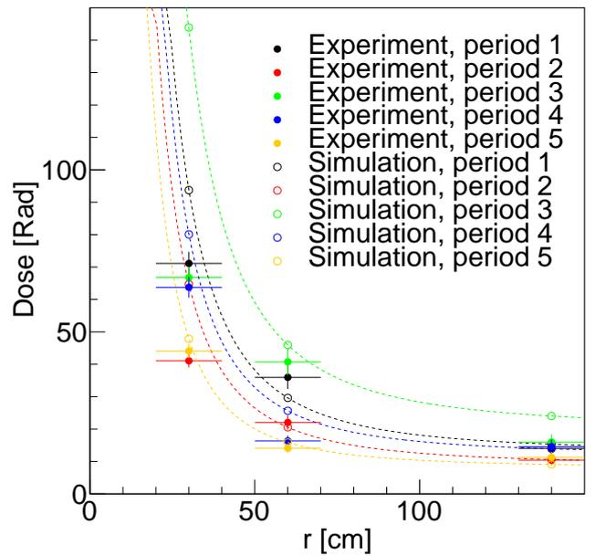
Figure 120: Integrated dose versus radius, for dosimeters located at  $z = 0$  cm,  $\phi = 45^\circ$  and for different time period. Each time period corresponds approximately to two weeks. Filled data points: experimental data. Open data points: simulation.
