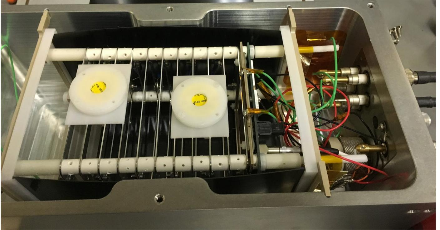
Figure 32: (color online) A photo of the inside of a TPC showing the internal calibration sources. The white containers with the yellow centers in the left half of the photo are the  $^{210}\text{Po}$  source holders. The source holder at the left of the photo is the “top” source; the source at largest drift distance, and the source holder towards the right of the photo, closest to the green wires, is the “bottom” source; the source at smallest drift distance.
