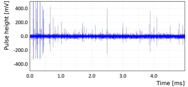
Figure 35: Typical scintillator waveform recorded by the PicoScope oscilloscope. Sampling intervals are 51.2 ns. The injected bunch arrives at  $t \sim 0.1 \text{ ms}$ , and noisy spikes are seen after the injection.
