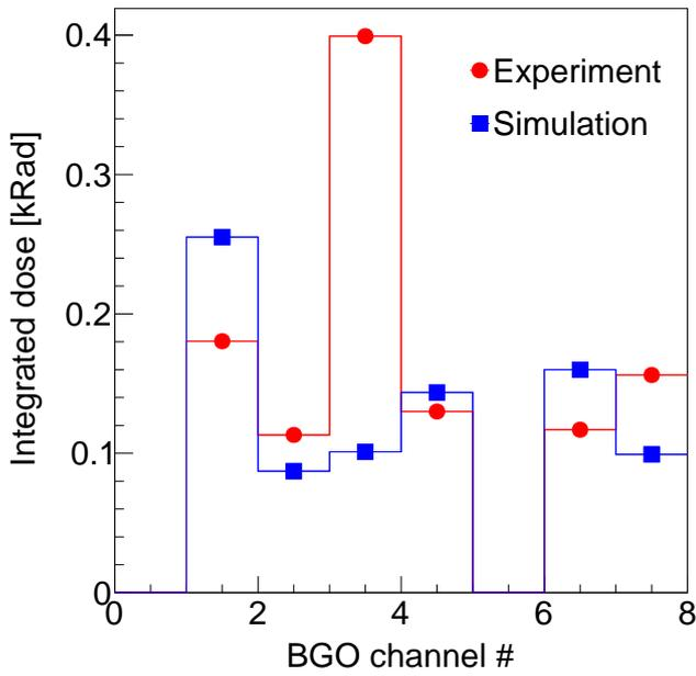
Figure 113: Measured and simulated integrated dose for each channel of the BGO detector system, with periods of injection excluded.
