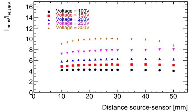
Figure 11: Example of the ratio of measured to predicted current  $G = I_{meas}/I_{FLUKA}$  for one of the three single-crystal diamond sensors, as a function of the distance  $d$ , for different HV bias values. The ratio increases with HV bias but it is stable for a given voltage applied.
