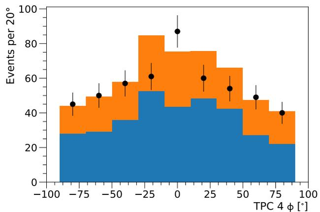
Figure 109: (color online) Azimuthal angle ( $\phi$ ) distribution for neutron event candidates in TPCs 3 (upper plot) and 4 (lower plot) for Monte Carlo and experimental LER data. The blue and orange histograms show the the stacked expectations for Touschek and beam-gas contributions obtained via rescaling the simulation, and the black points show the measured values in experimental data.
