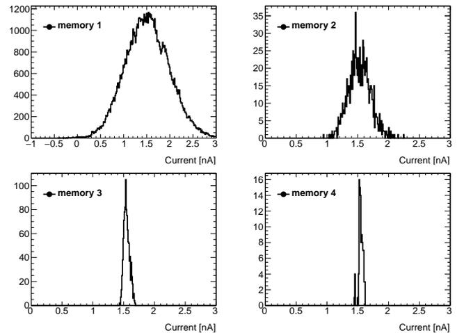
Figure 126: Histograms of data extracted from snapshots of the contents of the four buffer memories: (top left) first memory, 100000 entries, corresponding to a time interval of 1 s; (top right) second memory, 1000 entries, corresponding to the same 1 s; (bottom left) third memory, 1000 entries, corresponding to 50 s; (bottom right) fourth memory, 100 entries, corresponding to a time interval of 100 s.
