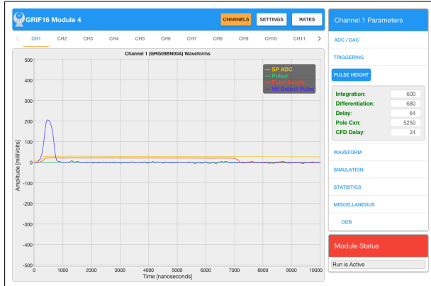
Figure 14: Screenshot of an example GRIF-16 digitizer User Interface for a single channel. The waveforms update in real time similar to a digital oscilloscope. The menus on the right allow the user to change parameters of the signal processing algorithms.
