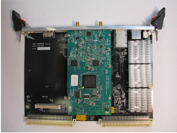
Figure 3: Photograph of the GRIF-4G module. The lower mezzanine card is removed.
