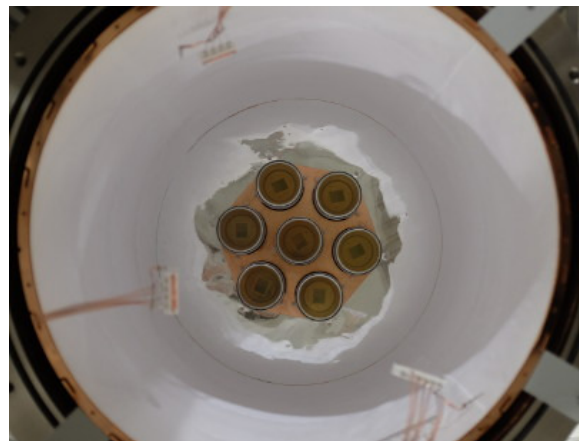
Fig. 11 Bottom PMT plate with 7 PMTs and copper cylinder. Plate and cylinder are covered by wavelength shifting Tetratex ® foil soaked in TPB [23].
