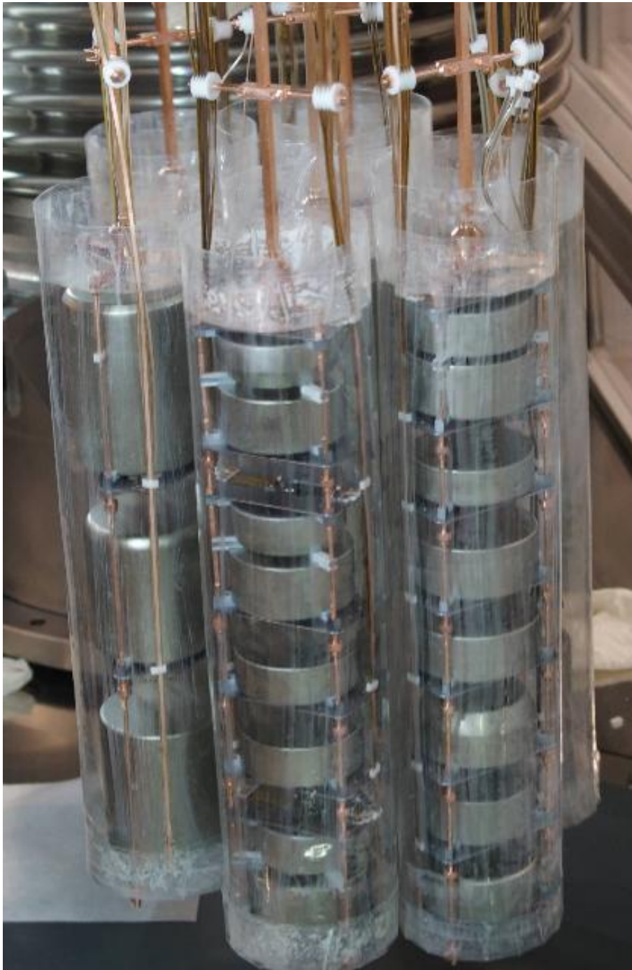
Fig. 31 Photo of GERDA Phase II detector array, showing from left to right string 2 with three semi-coaxial detectors, and strings 3 and 4 with eight BEGe detectors, respectively. Each of the seven strings is enclosed by a transparent mini-shroud.
