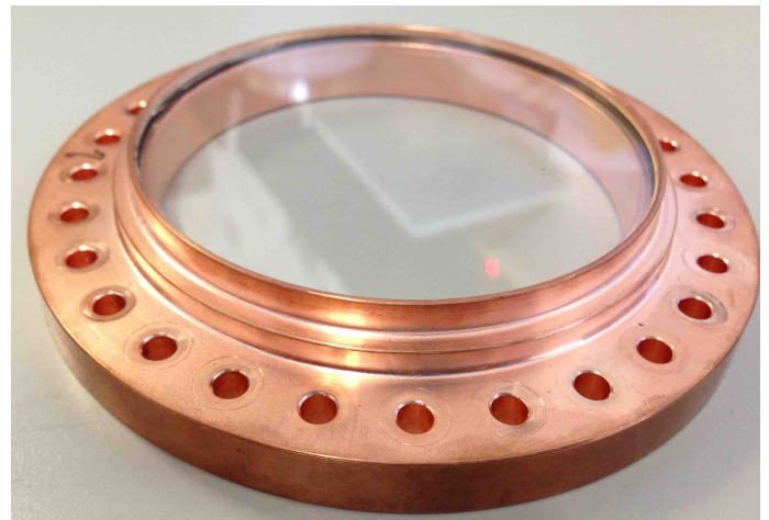
Figure 9: Scheme for the operation of PMTs in a helium-rich atmosphere ( top figure). The PMT itself remains at vacuum looking into the active volume through a crystalline quartz/sapphire window that can be coated with a wavelength shifter to maximize the light transmission. The crystal is welded to a metallic frame that can easily be mounted in a flange with a metallic sealing, avoiding helium diffusion into the PMT volume. The bottom figure shows one of the NEXT-NEW PMT protective windows. A similar concept can be applied for operation within a helium atmosphere using a metallic sealing for this frame.
