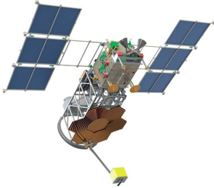
Figure 1: The TUS detector on board the Lomonosov satellite.
