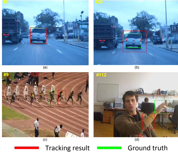
Figure 3: The tracking result with the model which does not use the loss function simultaneously considers tracking accuracy and bounding box quality.
