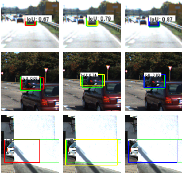
Figure 4. Comparison between SSD and RRC. Left column: results of SSD, failed to generate bounding box with IoU bigger than 0.7 to the groundtruth; Middle column: RRC, NMS over output 2 through output 6; Right column: RRC, NMS over output 3 through output 5.
