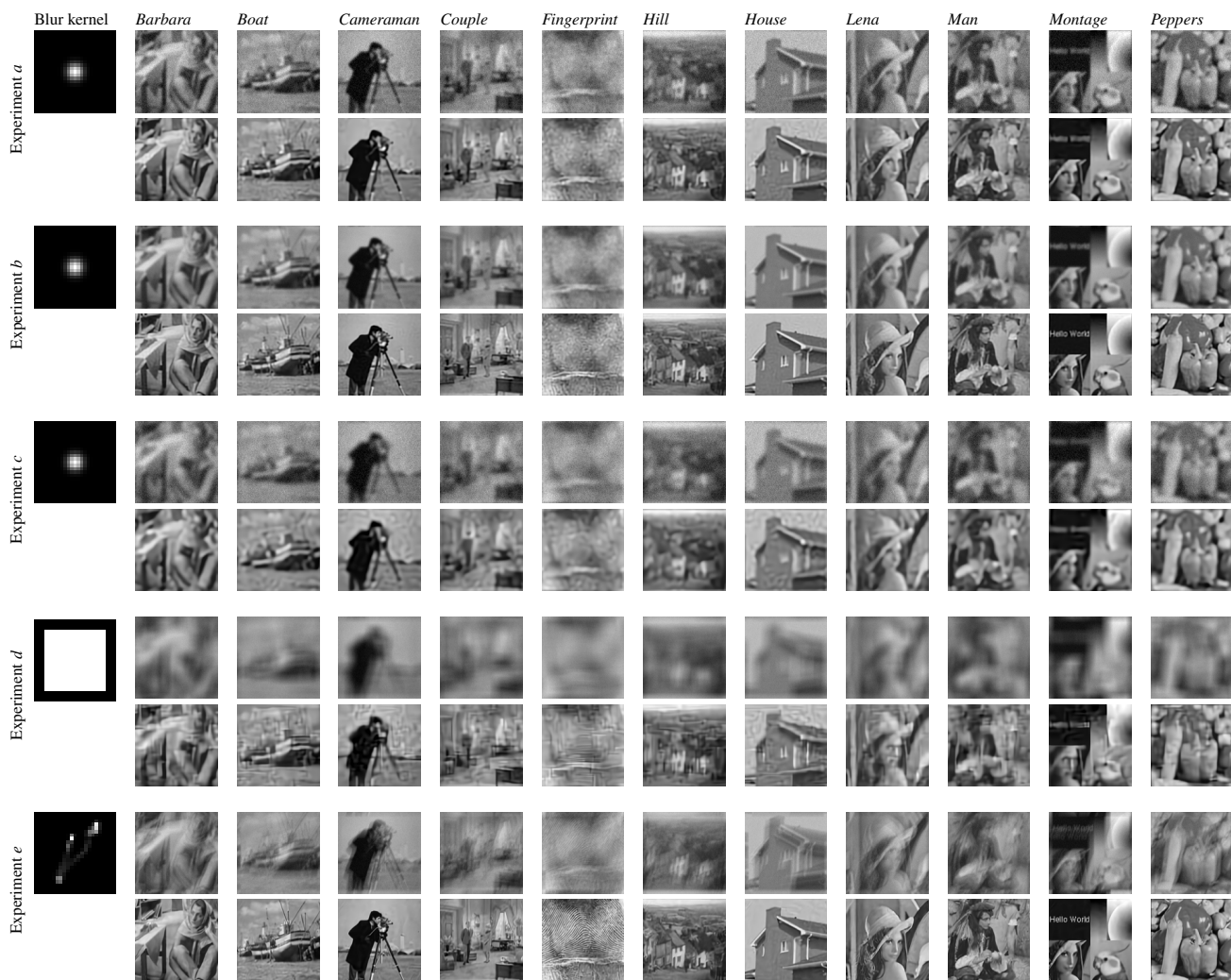
Figure 2: Our deconvolution dataset based on the experiments introduced in [35]. Each image ( 128 \times 128 pixels) is shown in its corrupted as well as by our approach reconstructed version. The deblurring was performed using the fixed denoising network trained on \sigma = 0.02 . To avoid boundary effects the images were cropped by 12 pixels. For visualization purposes we show enlarged versions of the different blur kernels.
