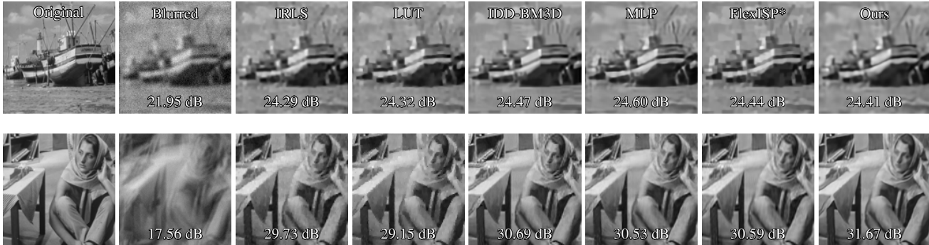
Figure 5: Visual comparison of different deconvolution methods on two out of 11 standard test images. The images Boat and Barbara were each corrupted with Gaussian noise ( \sigma = 0.04 , \sigma = 0.01 ) and a Gaussian blur (experiment a ) as well as a motion blur (experiment e ), respectively. Apart from FlexISP* and our result, all other images are taken from [19].
