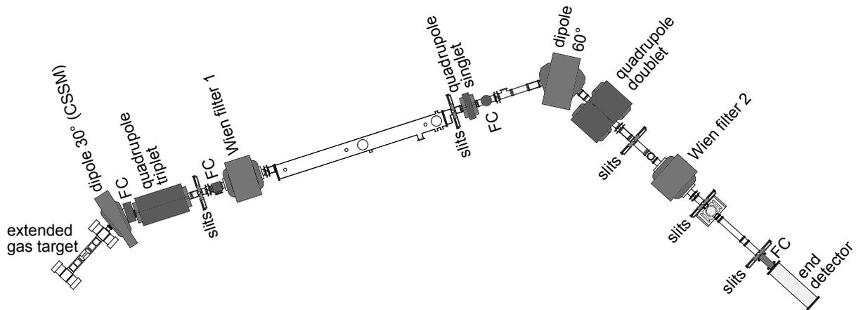
FIG. 1. Schematic view of the ERNA recoil separator.
