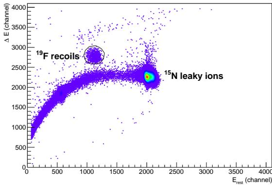
FIG. 7. Sample ICT  $E_{\text{rest}}-\Delta E$  spectrum for ions identification and counting, collected at  $E_{^{15}\text{N}} = 7.06$  MeV.
