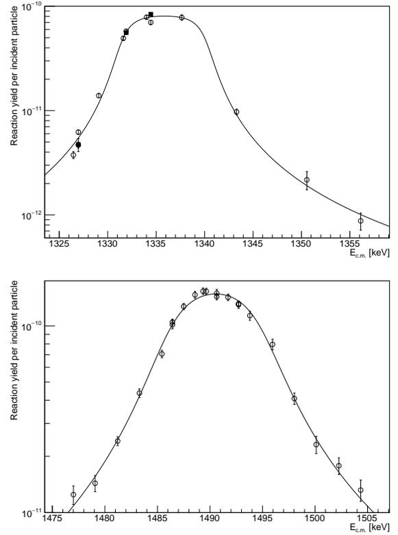
FIG. 8. Reaction yield per incident projectile observed for the two broad resonances at 1323 keV and 1487 keV, top and bottom respectively. Open circles and filled squares indicate measurements of recoils in the 4+ and in the 3+ charge state, respectively.
