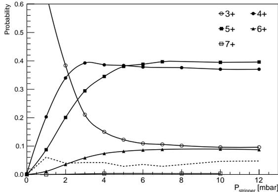
FIG. 4. Charge state probability of  $^{19}\text{F}$  ions as a function of the Ar post-stripper inlet pressure  $P_{\text{stripper}}$  at 5.0 MeV beam energy. Lines connecting the points are to guide the eye only. The dotted line represents the unmeasured current at this energy, due to non accessible 1+, 2+ charge states and further charge exchanging in the CSSM chamber, see text for details.
