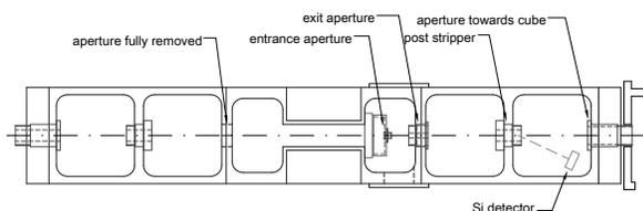
FIG. 2. Schematic top view of the modifications to the extended gas target chamber. The relevant parts discussed in the text are indicated, for further details see Ref. [20].
