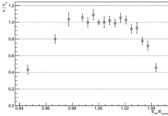
FIG. 6. Ratio of the observed yield  $Y$  with respect to the central yield  $Y_0$  of the  $E_{\text{c.m.}} = 1323$  keV resonance as a function of the energy set for the separator.
