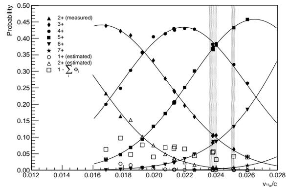
FIG. 5. Charge state probability of  $^{19}\text{F}$  ions emerging from the target as a function of velocity. Filled symbols are experimentally determined values, while empty symbols are estimated values for the unmeasured 1+, 2+ charge states and for the further charge exchanging in the CSSM chamber, see text for details. Curves through points are uncorrelated Gaussian fits. Vertical shaded areas indicate the energy intervals where cross section measurements were performed.
