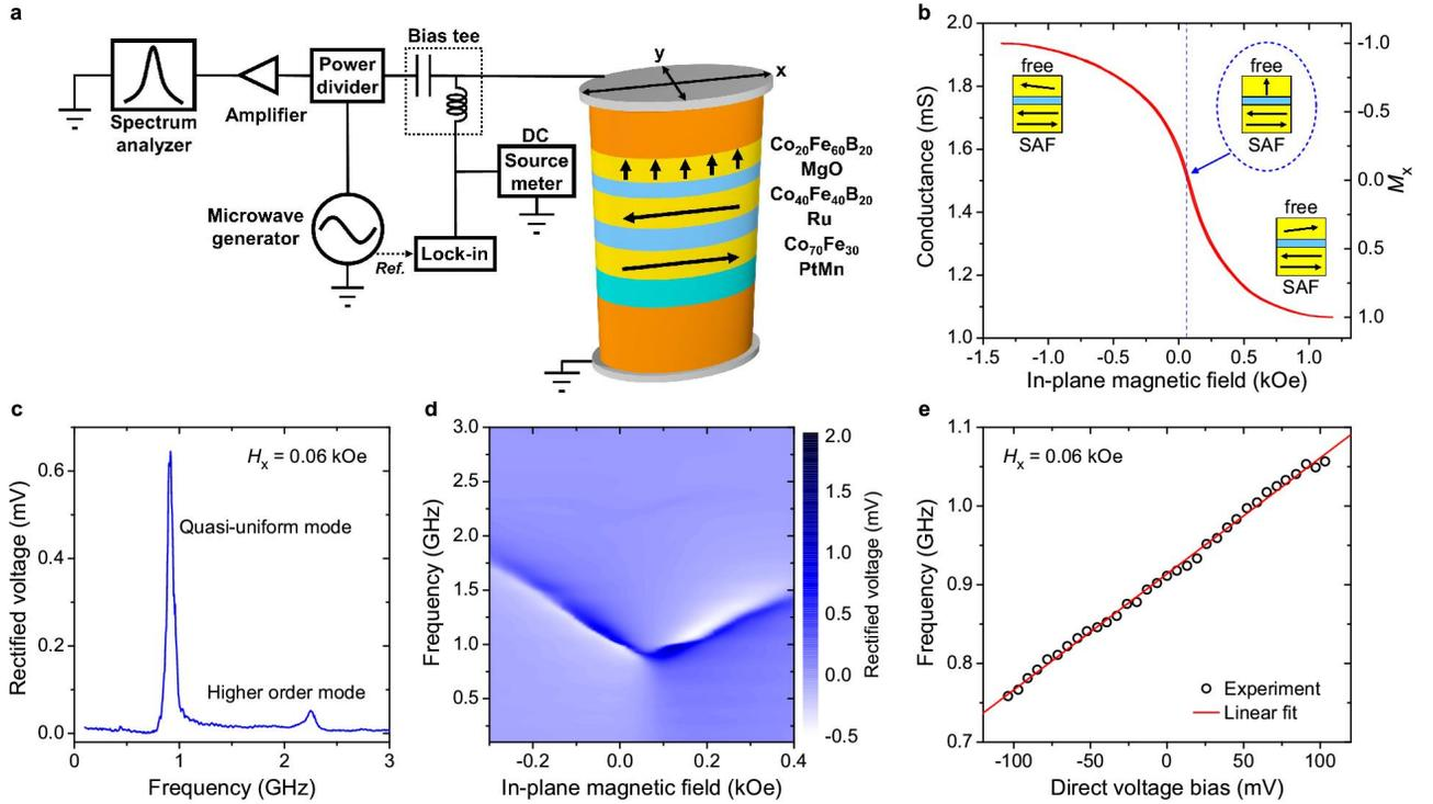
**Figure 1. Measurement setup and MTJ characterization.** **a**, Schematic of experimental setup for DC and microwave characterization of MTJ. **b**, MTJ conductance as a function of in-plane magnetic field  $H_x$  applied parallel to the MTJ long axis. **c**, ST-FMR spectrum of the MTJ at  $H_x = 0.06$  kOe. **d**, Dependence of ST-FMR spectra on  $H_x$ . **e**, Quasi-uniform mode frequency versus direct voltage bias  $V_{dc}$  measured at  $H_x = 0.06$  kOe.
