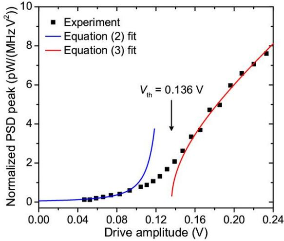
**Figure 3. Parametric resonance threshold.** Normalized peak amplitude of PSD,  $P(f_{\text{pr}}/2)/V_{\text{ac}}^2$ , measured at parametric resonance as a function of the parametric drive amplitude  $V_{\text{ac}}$ . Best fits of equation (2) and equation (3) to the data (solid lines) give the parametric resonance threshold voltage  $V_{\text{th}} = 0.136$  V.
