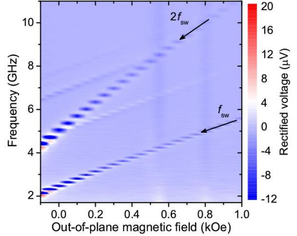
**Figure 4. Parametric resonance in ST-FMR.** ST-FMR spectra of an MTJ with out-of-plane SAF and free layers measured as a function of out-of-plane magnetic field. Resonance at twice the quasi-uniform mode frequency arises from parametric excitation of the quasi-uniform mode.
