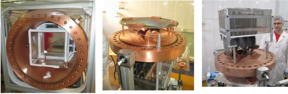
Figure 2. Different views of the TRES-DM setup showing the field cage and cathode, Micromegas readout and electronics.
