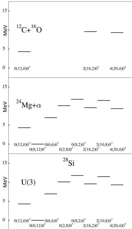
FIG. 5. The spectra of the  $0^+$  states in the  $^{28}\text{Si}$  nucleus and in its  $^{24}\text{Mg}+^4\text{He}$  and  $^{16}\text{O}+^{12}\text{C}$  clusterisations, as predicted by the Hamiltonian of the multichannel dynamical symmetry [7]. The states are characterised by the  $n(\lambda, \mu)K^\pi$  quantum numbers, where  $n$  is the major shell excitation, and  $(\lambda, \mu)$  refers to the  $\text{SU}(3)$  representation i.e. the quadrupole deformation.
