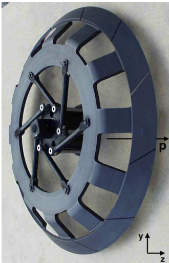
FIG. 6. Picture of the Target E wheel used for surface muon production at PSI. The proton beam impinges on the outer rim as shown by the arrow. In order to radiatively cool the target, the wheel rotates with a frequency of 1 Hz.
