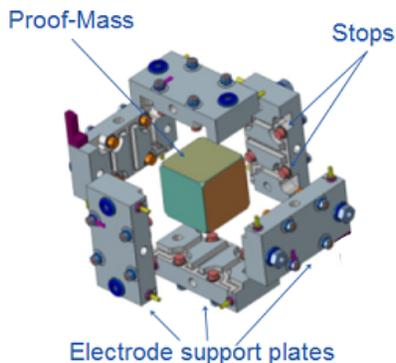
FIG. 17. **Sensor core of the external accelerometer.** The figure shows test mass and electrode housing. Size of sensor core:  $\leq 10 \times 10 \times 10 \text{ cm}^3$ , mass:  $\leq 2 \text{ kg}$ . Image credit: ONERA.
