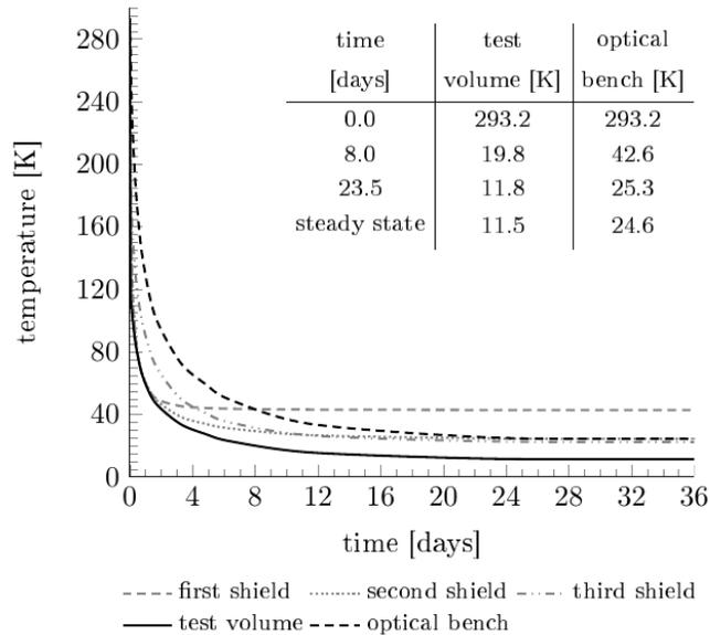
FIG. 23. **Cool-down of parts of the thermal-shield structure over time.** Starting from room temperature, the optical bench reaches steady state after about 25 days. Due to its small volume and low heat capacity, the test volume temperature drops more rapidly. Figure from Ref. [38].
