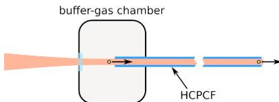
FIG. 18. **Transfer of particles through hollow-core photonic-crystal fiber (HCPCF).** After loading and characterization of a nanoparticle (indicated by a green dot) inside a buffer-gas chamber, the particle is optically guided into and along a HCPCF outside the spacecraft.
