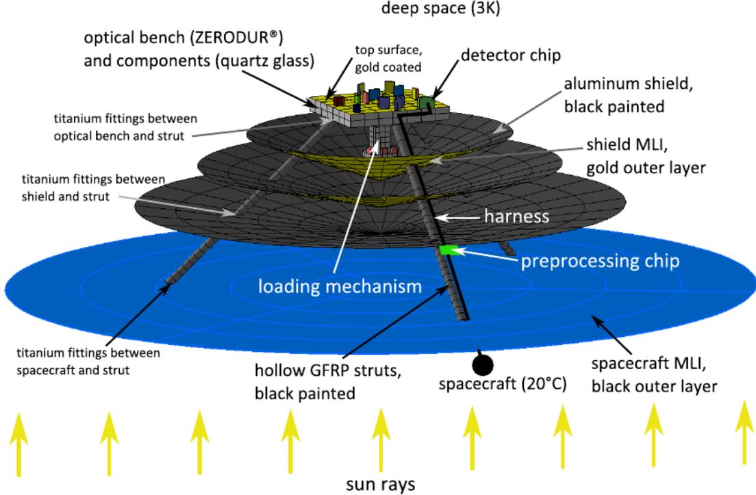
FIG. 13. **CAD drawing of heat-shield geometry.** The structure is attached to the spacecraft facing away from the sun. Three glass-fiber reinforced plastic (GFRP) struts hold three consecutive shields isolating the optical bench from the spacecraft surface (Image source: Ref. [38]).
