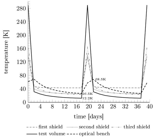
FIG. 22. **Temperature of the heat-shield structure in HEO configuration.** Close to perigee, the thermal-shield structure heats up and then needs more than two weeks to cool down again to fulfil the requirements of MAQRO. Figure from Ref. [38].
