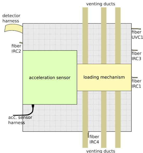
FIG. 15. **Bottom view of the optical bench.** The image illustrates where venting ducts could be placed to minimise the amount of buffer gas potentially leaking to the experimental region. The figure also shows the position of the external acceleration sensor and fibers from the top of the optical bench.
