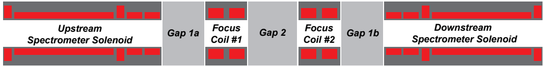
Figure 10. Generic schematic for MICE Final Cooling Demonstration, containing three gaps into which RF cavities and/or absorbers may be placed.
