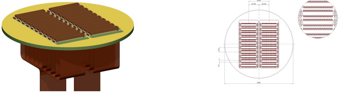
FIG. 80: Signal feedthrough and connectors from the CRP (left) 3D view (right) 2D top view.
