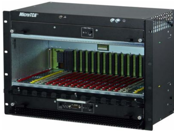
FIG. 76: Picture of the Schroff 11850-015 8U shelf.
