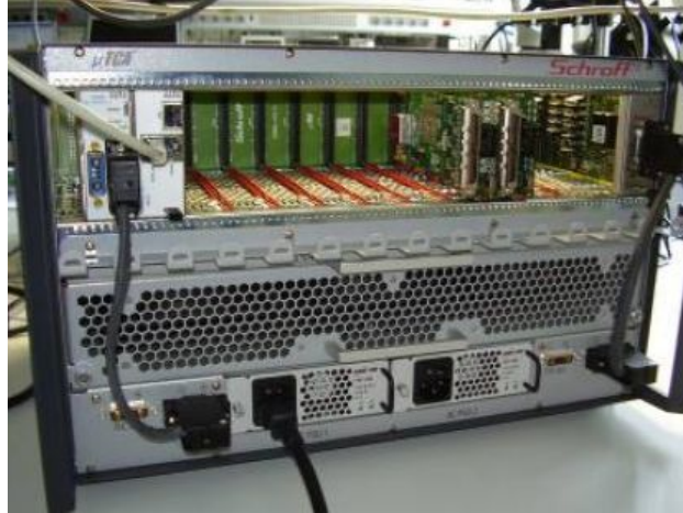
FIG. 67: Picture of a micro-TCA crate containing DAQ boards with 32 ADC channels/board as developed in 2010.
